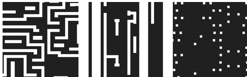
Fig. 1 From left to right: Illustrative examples of 1024 nm × 1024 nm tiles from metal 1 (M1), metal 2 (M2), and contact array (CA) layers, respectively. Note that they exclusively contain rectilinear polygons.
