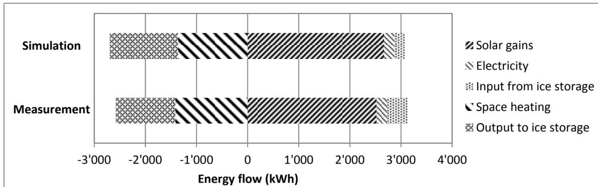
Figure 4: Comparison of simulated and measured energy flows in the heating system of the pilot plant for 17 days in April 2013.
