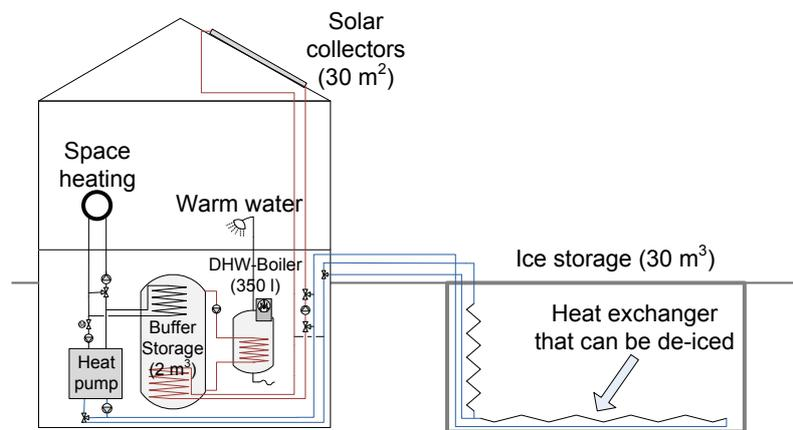
Figure 1: Simplified hydraulic scheme of the simulated heating system with ice storage and  $SPF_{sys}$  of 6 and sizes of the main components for a single family house.
