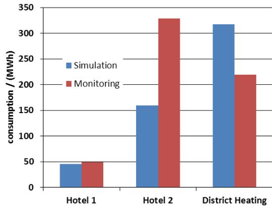
Figure 3: Simulated and monitored consumption for space heating and domestic hot water for the first year of operation for three example energy systems
