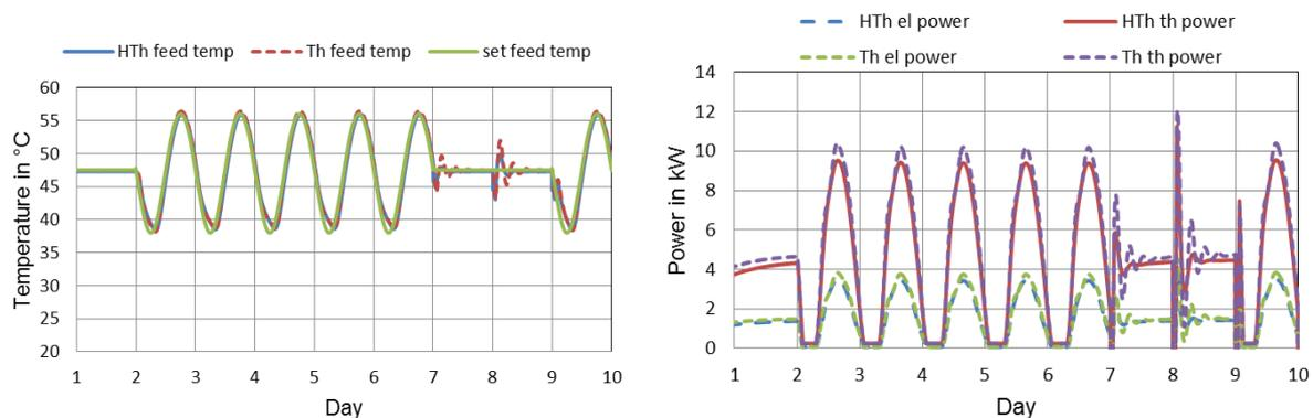
Figure 4: Comparison of the feed temperature and energy output
