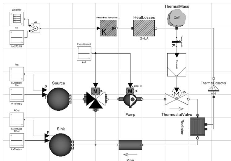
Figure 4: Scheme of the simple heating circuit model
