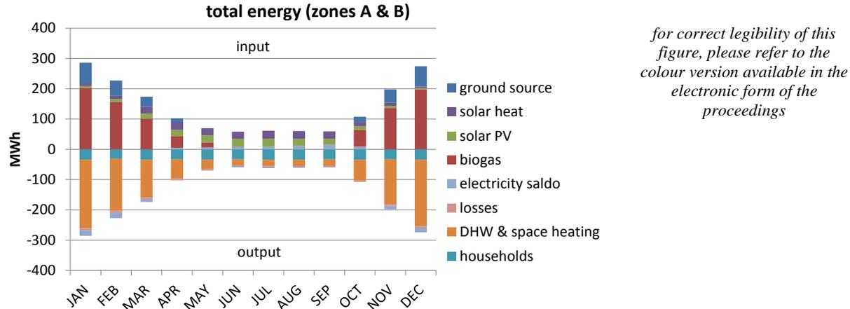
Figure 4: Monthly balance of all energy inputs and outputs of the whole development area.
