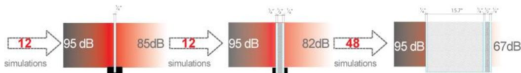
Figure 4: Progression from sealed single-glazed facades to sealed double-skin facades based on improved sound transmission loss from analysed simulations.
