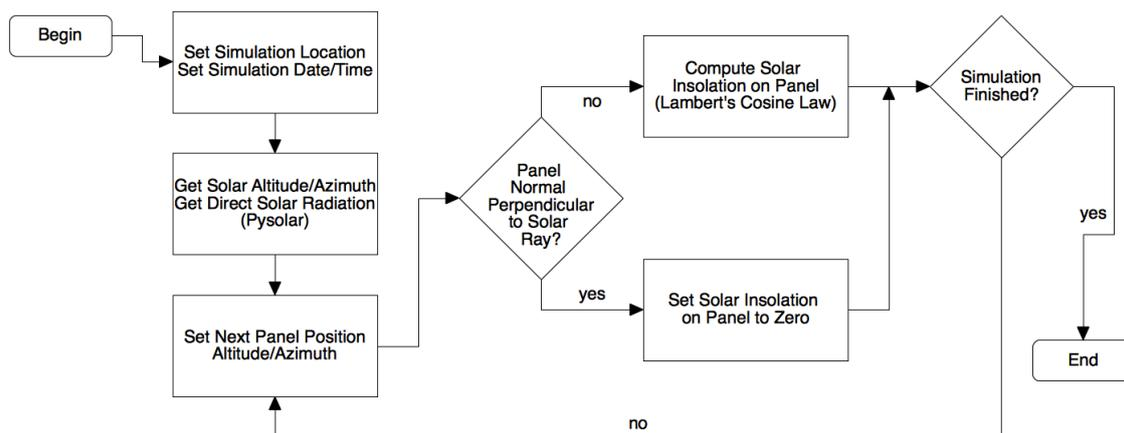
Figure 3: Flow diagram of the lightweight solar insolation framework (LSIF).
