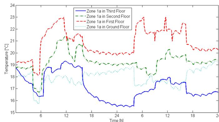
Figure 5: Air temperature in zone 1a of each floor
