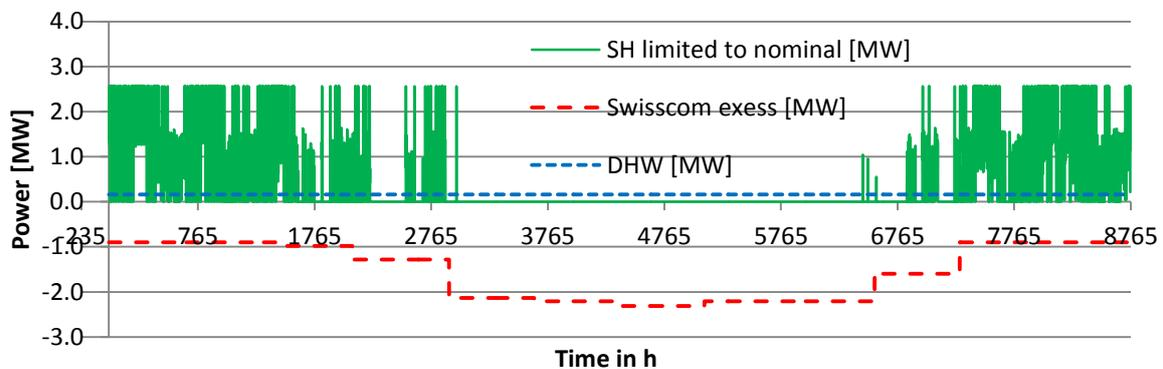
Figure 2: Estimation of the heating and regeneration loads at the “Grünmatt” ground storage after the first construction phase. (Coloured graph only available in the digital version of the paper)
