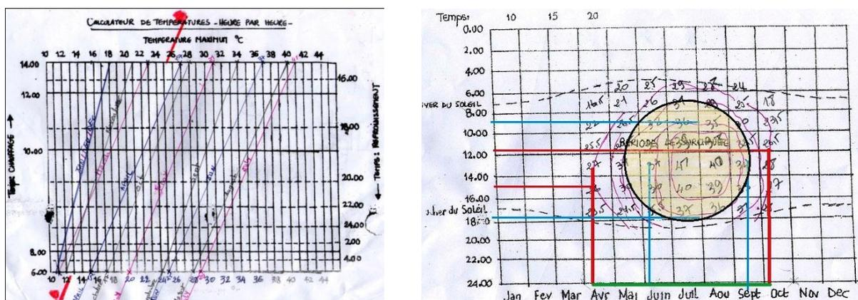
Figure 2(a): Hourly temperature calculator. (b): Ziban's matrix temperature per months and hours. Source : S. Szocolay, (1979) [8]
