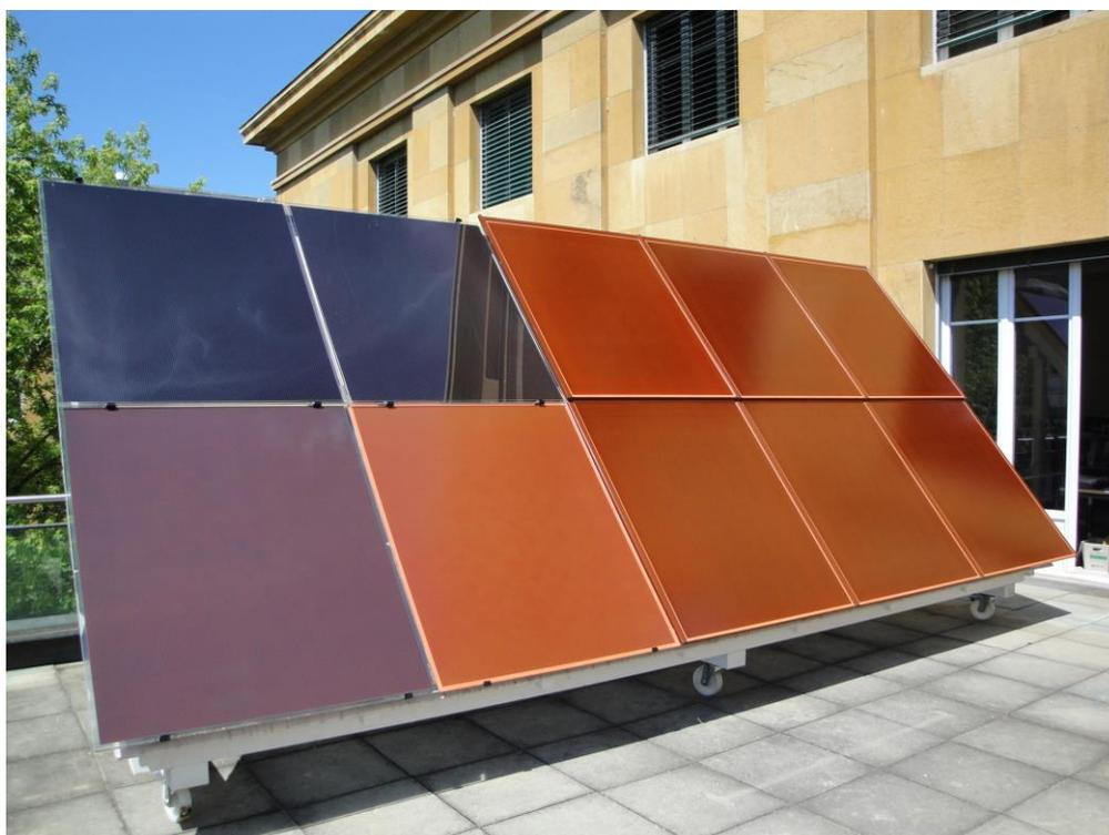
*Fig. 4: Demonstration roofs with the new orange colored PV modules*
