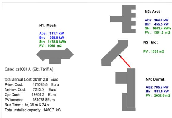
Figure (4): optimized cooling system obtained for Case study 1 for: Tariff A.
