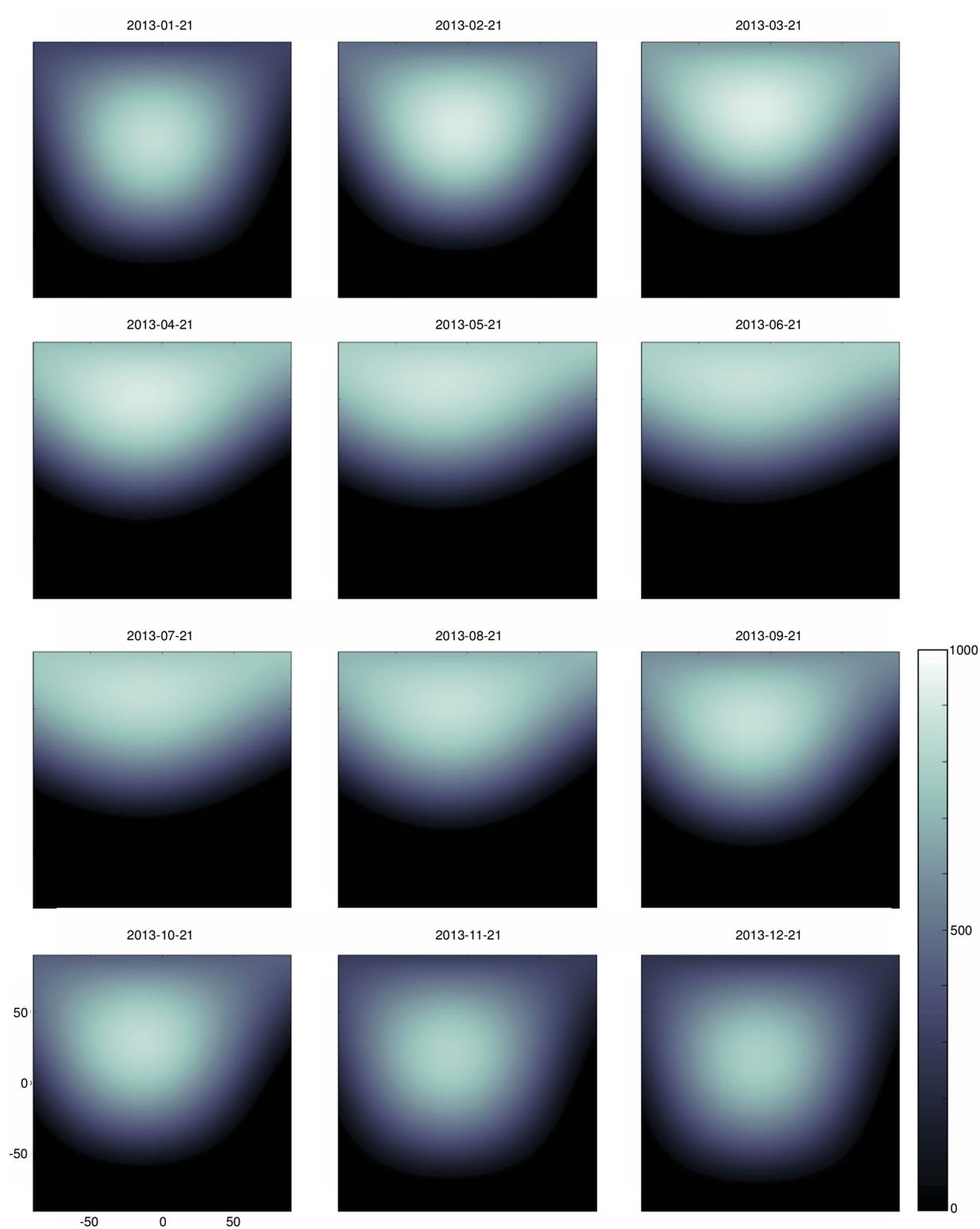
*Figure 2: Scatter plots of solar scan results at 12:00:00 on the 21<sup>st</sup> day of each month. The x-axis represent the horizontal orientation of the panel and the y-axis represent the vertical orientation of the panel. Both x and y axes have a range from -90 to 90 degrees. Each plot is comprised of 32,400 data points. The colormap scale represents  $W/m^2$ .*
