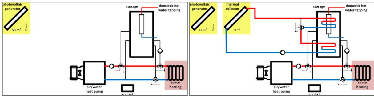
Figure 1 System and hydraulic scheme of system 1 (left) and system 2 (right)
