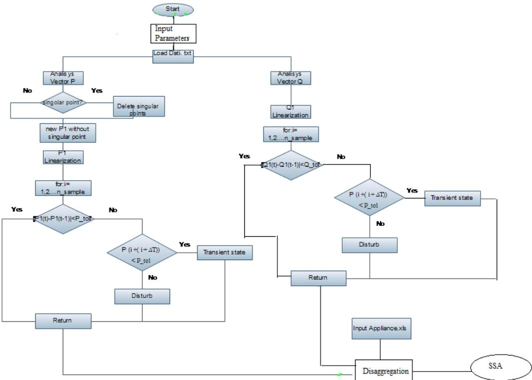
Figure 3: Flowchart of the proposed NILM algorithm
