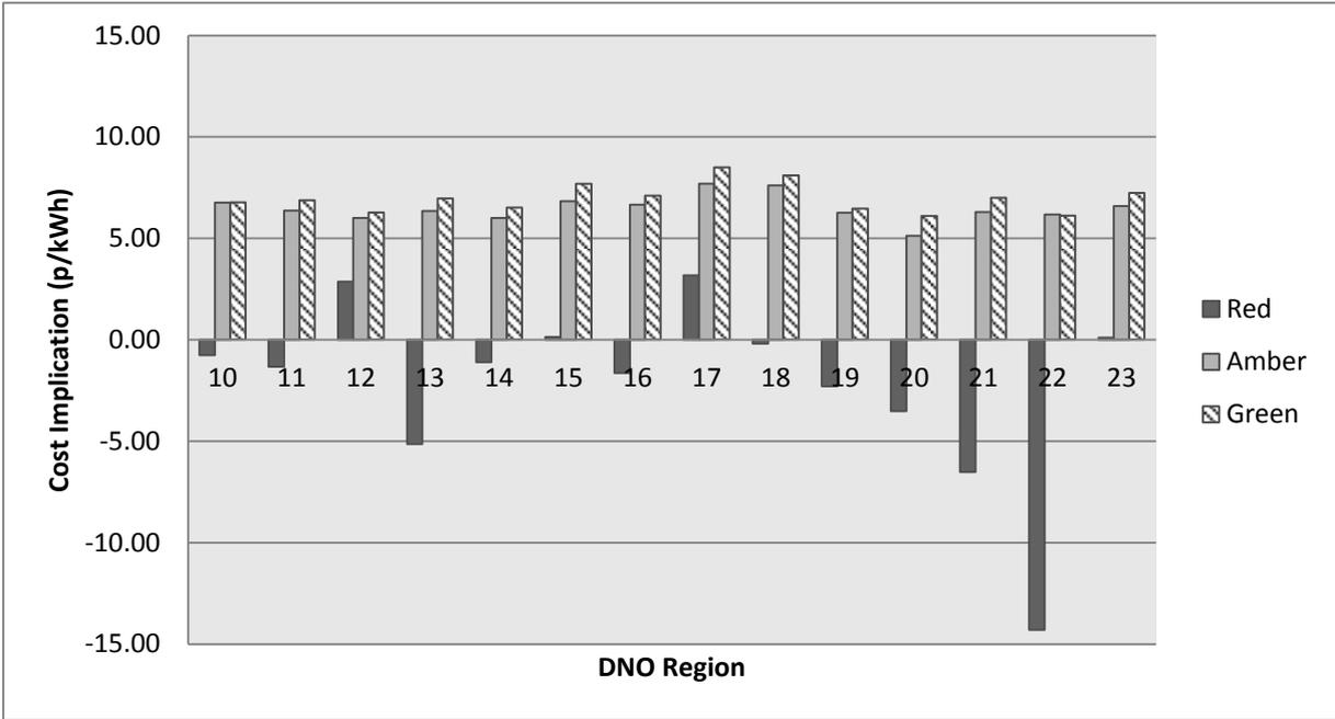
Figure 1: Cost Implications of Diesel Generators at Different Charging Periods (Low Voltage)
