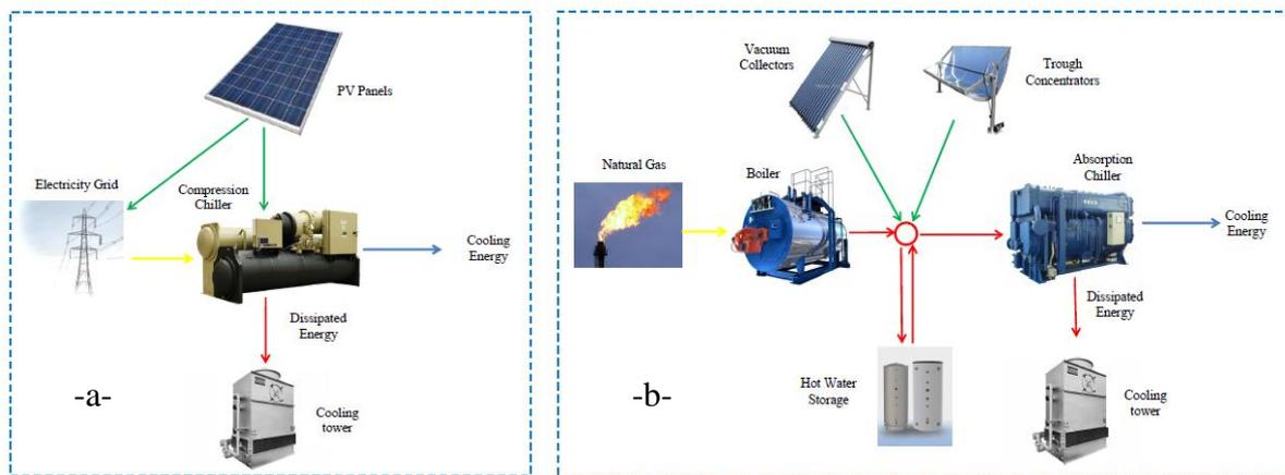
Fig. (1a & b): Configuration options for the cooling energy generation plant on site (i).
