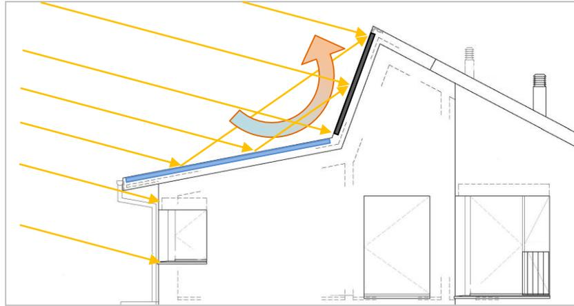
Figure 2: Mirror effect on the photovoltaic field (blue, 11° inclined) onto the thermal collectors (black, 70° inclined) for low solar elevation (15 – 25°). This yields a 20% increase in the solar thermal gain during wintertime. In addition, the rising warm air from the PV field (round arrow) reduced the losses of the thermal field (in winter and summer) and hence increasing the yield furthermore.
