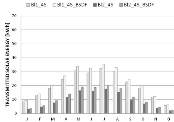
Figure 7: Monthly transmitted solar energy through window for B11\_45 and B12\_45.
