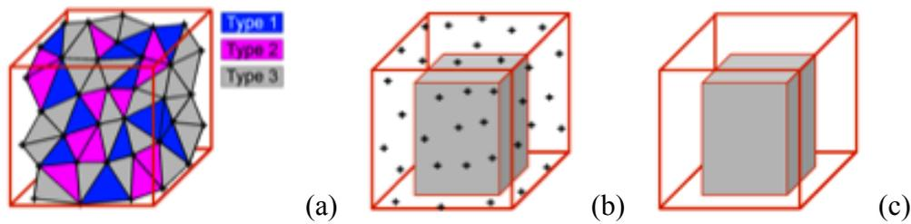
Figure 2: Envelope description. a – triangular facets and their types; b – control points of the geometry; c – internal and external constraints restraining control points positions
