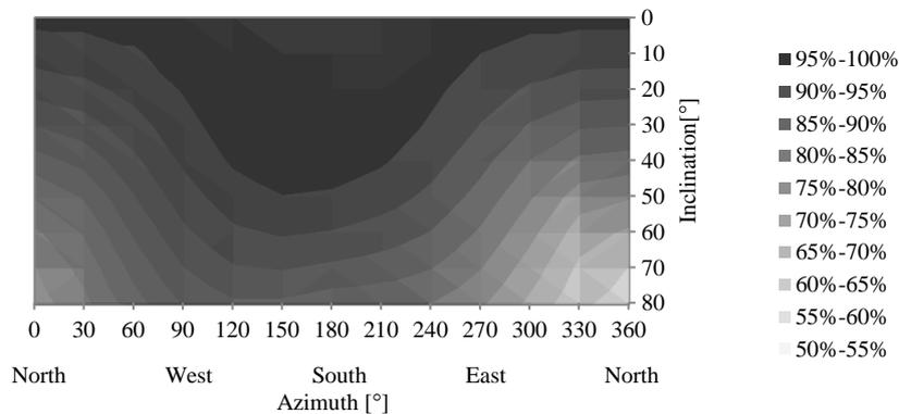
Table 1: Relative PV/T surface efficiency (thermal yield in summer). The system configuration allows more flexible placement compared to installations, which focus on the yearly gains.
