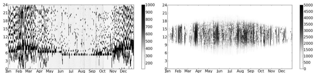
Figure 4: Carpet Plot for electric consumption (left) and PV generation (right) for the floating demo-building (time: CET, latitude: 51.7°)
