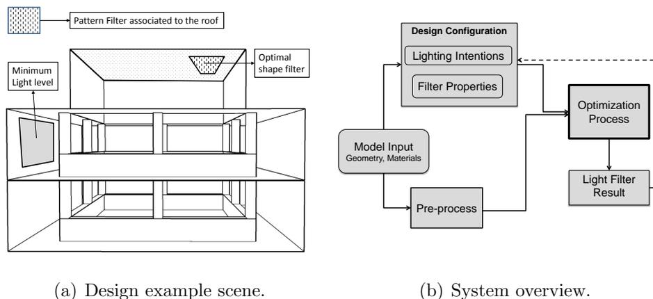
Figure 2: From a given design specification and filter pattern (a), our pipeline uses an optimization process to compute the optimal filter shape (b).
