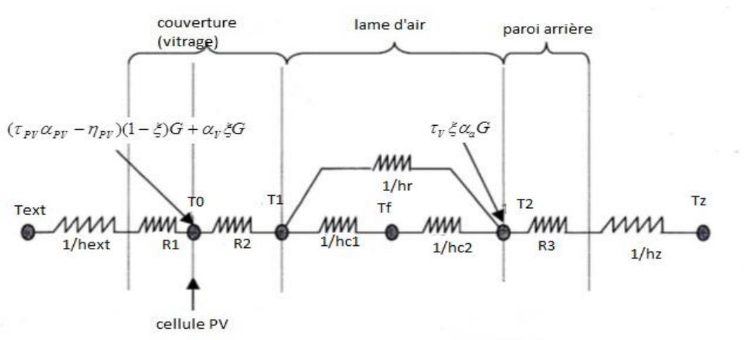
Figure 1: Nodal model of a ventilated PV double skin façade
