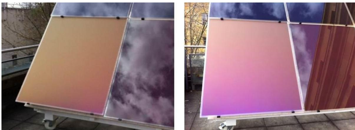
*Fig. 4: Orange glass panes laminated on real-size PV modules (1.10 x 1.30 m<sup>2</sup>) on which strong angular dependency of the color is observed.*
