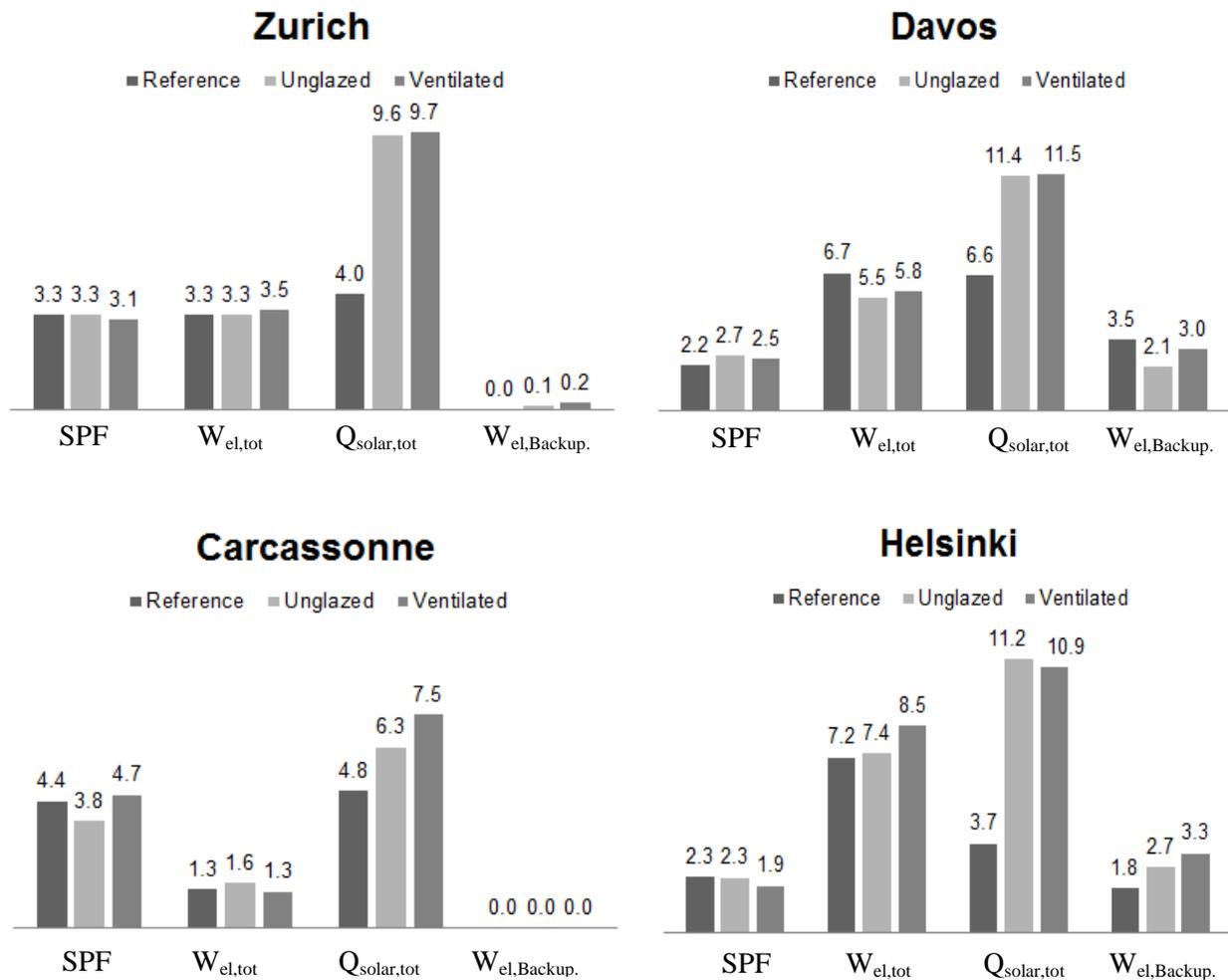
Figure 4: Result summary of the comparison of all three systems, all energies in MWh
