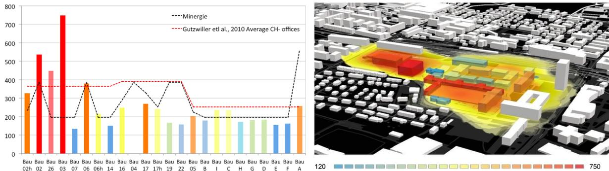
Fig. 1 2D and 3D Visualization of energy performance values end-uses for room heating, domestic hot water and humidification ( $\text{MJ}/\text{m}^2\cdot\text{yr}$ ) in comparison to Minergie standard  $Q_h \leq 90\% Q_{hlim}$  and the regional average after Guzwiler et al., 2010 [11]
