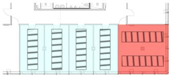
Figure 4: Floor plan detail: 2 zones with position of radiant panels.
