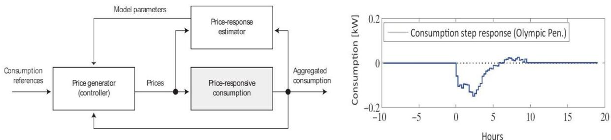
Figure 5: (a) Schematic of a system used to control electricity consumption in buildings using price signals and (b) Consumption response when the electricity price increases at hour 0.
