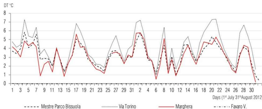
Figure 5. Mean night (9pm-3am) temperatures differences  $\Delta T$  (°C) 1<sup>st</sup> July-31<sup>st</sup> August 2012 for three weather stations with respect to Favaro Veneto station.
