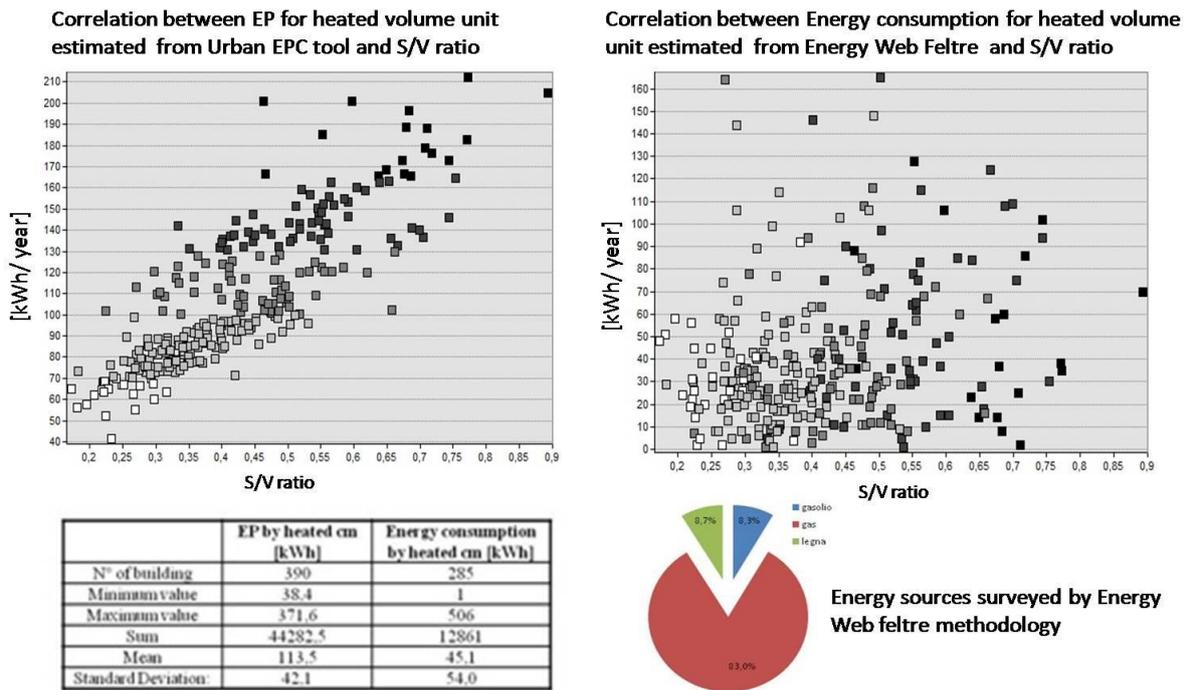
Figure 4: Comparison between theoretical EP need and end-use consumption
