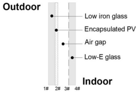
Fig. 1: Schematic of the PV window.
