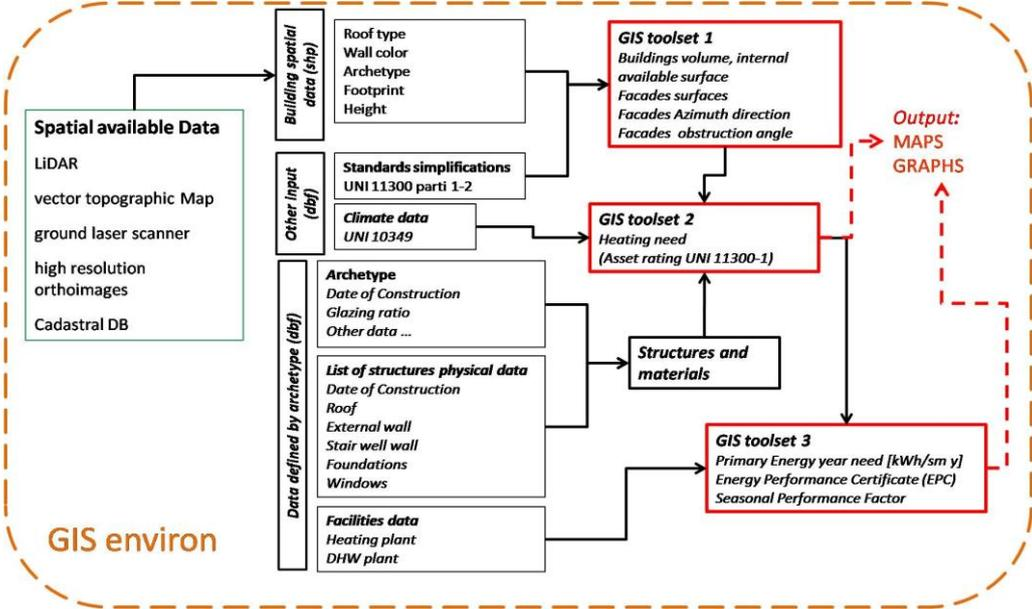
Figure 2: "Urban EPC" methodology logic schema and workflow
