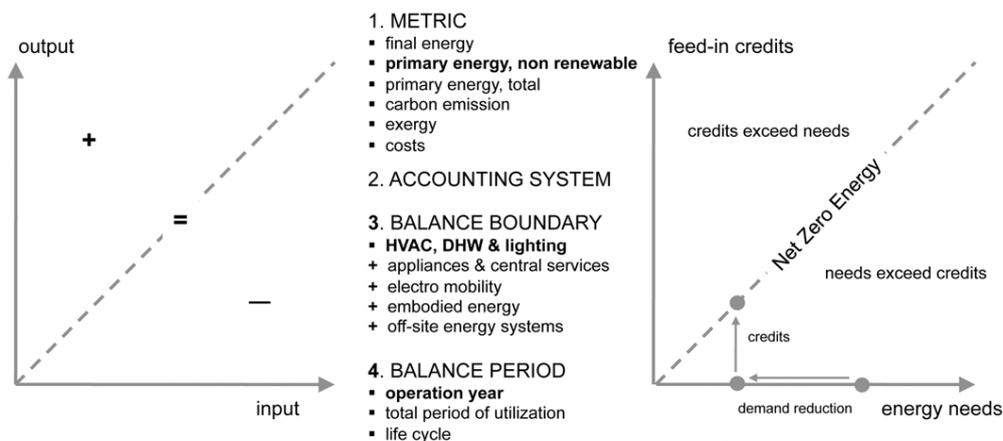
Figure 2: Schematic input/output balance of a building (from [1]). By defining a metric, an accounting system, the boundaries for the energy balance and a balance period a building (or district) can be evaluated. By applying efficiency measures a demand reduction is realized, covering the remaining energy needs with renewable sources leads to a net zero balance.
