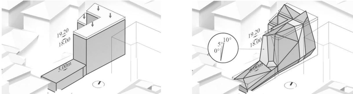
Figure 1. Comparison of the maximum allowable volume (*Vol.0*), initial volume (*Vol.A*) (on the left) and solar optimized volume (*Vol.B*) (on the right).
