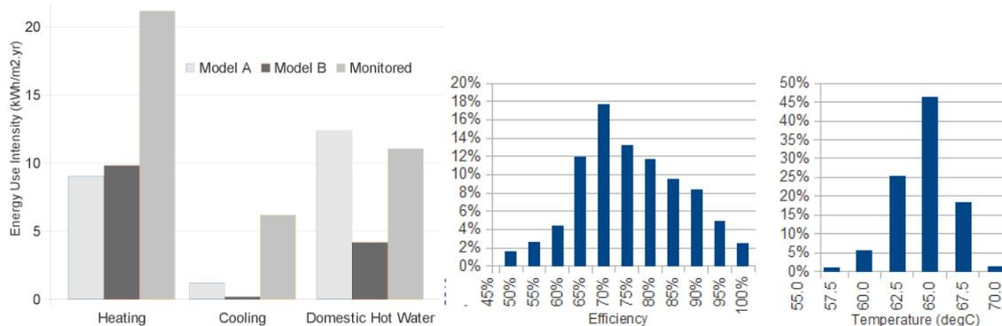
Figure 4: Comparison of (a) modelled and monitored sub-system EUIs and (b) frequencies of boiler efficiencies and water return-to-boiler temperatures measured at 15 minute intervals during operating period.
