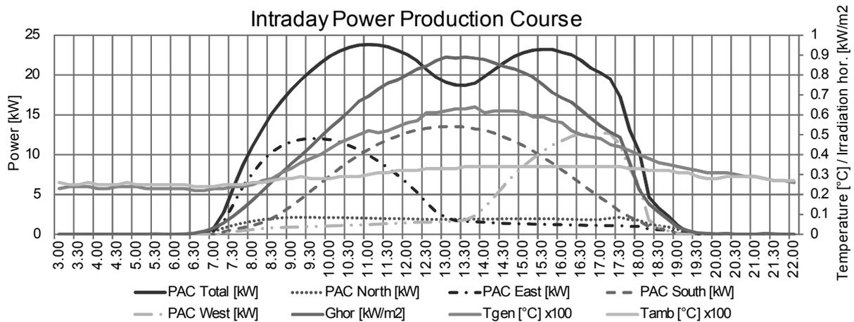
Figure 2: Daily course of AC power (total, east, south, west) superimposed by the generator and ambient temperature
