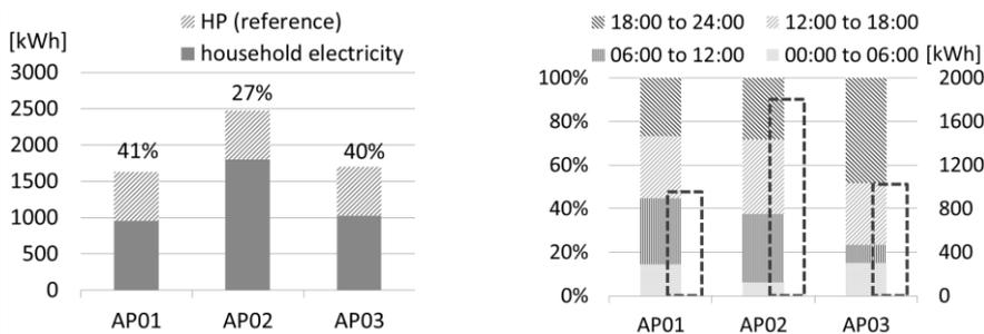
Figure 8: Comparison of different electric consumption-profiles from different households (size: 2 – 4 inhabitants).
