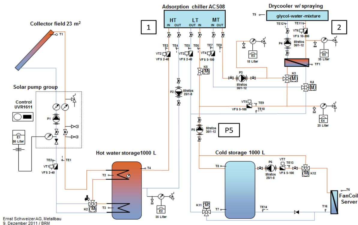
Figure 1: Schematic of the solar thermal driven 8kW ACS08 Silica Gel-H<sub>2</sub>O adsorption cooling machine of SORTECH AG (1). The heat rejection sub-system of the solar cooling system (2) can be used in the server room free-cooling mode (schematic: E. SCHWEIZER AG).
