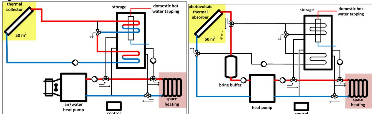
Figure 2 System and hydraulic scheme of system 3 (left) and system 4 (right)
