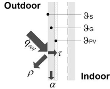
Fig. 2: Detailed scheme for solar radiation balance.
