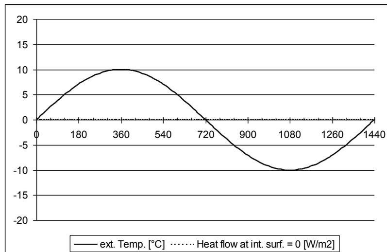
Figure 1 Concrete wall: heat flow rate through the internal surface [ $W/m^2$ ] (dotted thin line) and outdoor temperature in  $^{\circ}C$  (continuous thick line) over the period of one day (x-axis). In this case the heat flow rate equals zero.
