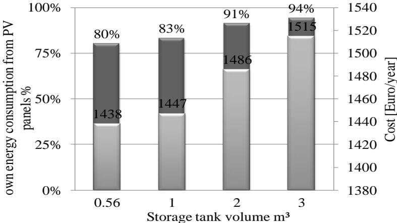
Figure (2): Own energy consumption from PV panels and energy cost balance with different storage volumes
