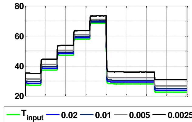
Figure 2 : Outlet temperatures for  $\dot{m} = 0.02 \text{ kg/s}$  ;  $\dot{m} = 0.01 \text{ kg/s}$  ;  $\dot{m} = 0.005 \text{ kg/s}$  and  $\dot{m} = 0.0025 \text{ kg/s}$  ; with  $T_{inlet} = 27.2^\circ\text{C}$  ;  $T_{inlet} = 37.2^\circ\text{C}$  ;  $T_{inlet} = 47.2^\circ\text{C}$  ;  $T_{inlet} = 57.9^\circ\text{C}$  ;  $T_{inlet} = 68.5^\circ\text{C}$  ;  $T_{inlet} = 28.1^\circ\text{C}$  and  $T_{inlet} = 22.5^\circ\text{C}$
