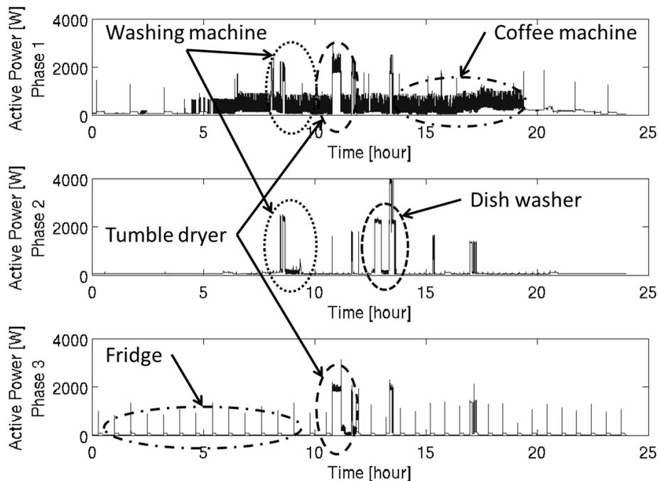
Figure 2: Typical 24 hour recording (active power, three phases).
