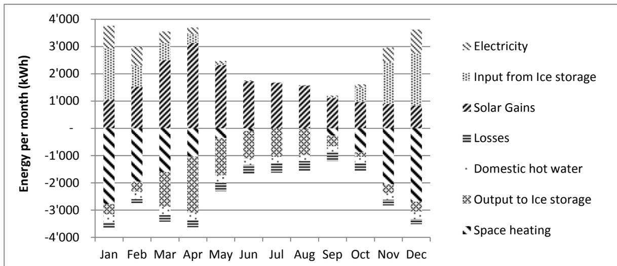
Figure 2: Simulated energy flows per month of the heating system with ice storage reaching an  $SPF_{sys}$  of 6 in a single family house with space heating demand of 14 MWh per year.
