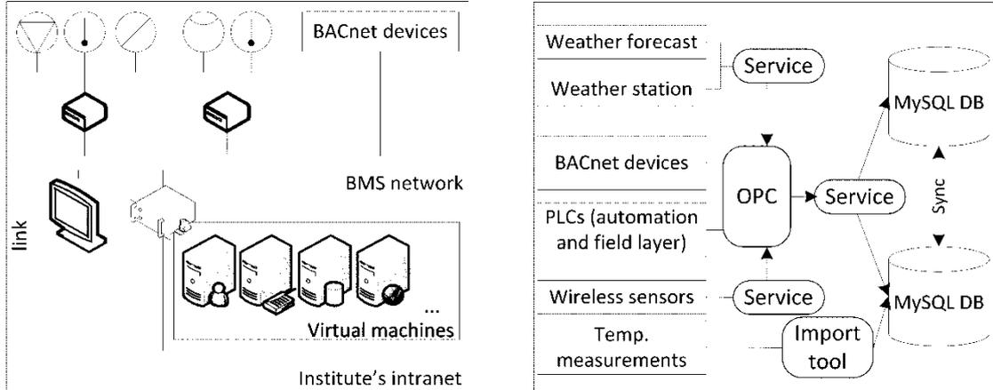
Figure 2: left: Building automation infrastructure with cloud server and link to the institute’s intranet; right: Schematic of the data logging and storage system
