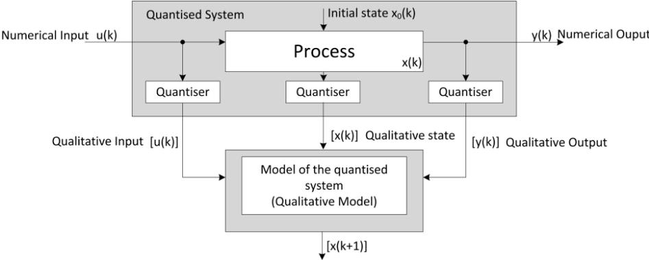
Figure 2: Supervision of a quantised system, based on [6].
