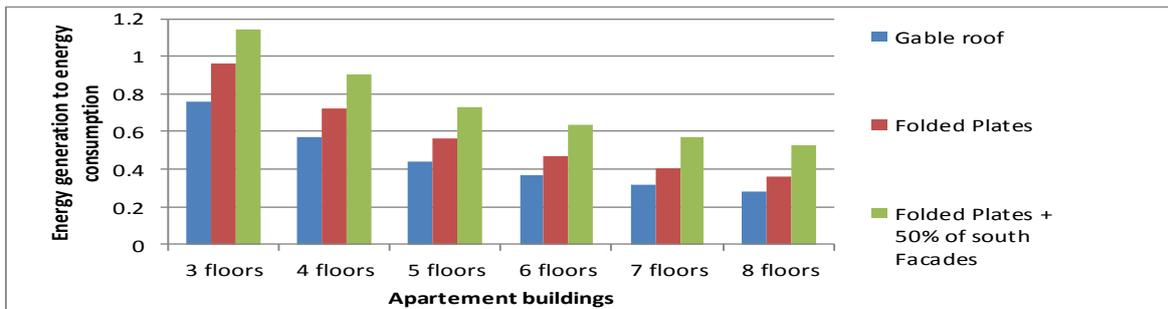
Figure 5, Comparison of generation to consumption for different design options.
