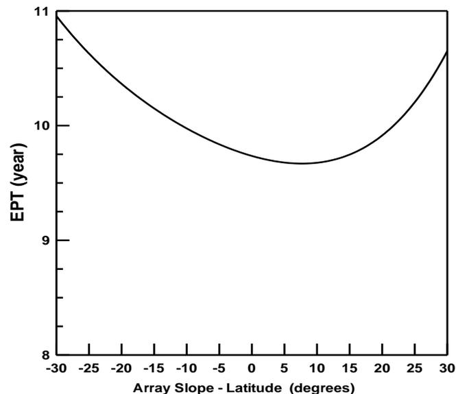
Figure 1: Variation of EPT with tilt angle at fixed azimuth angle (azimuth= $0^\circ$ )
