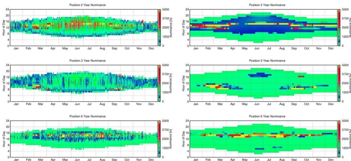
Figure 3: Heat maps of illuminance contributed from reflected daylight received at critical positions 2, 3 and 6 using Zurich weather data and CIE clear sky model.
