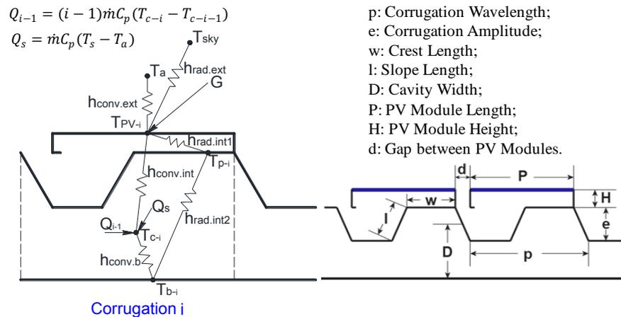
Figure 1: Thermal network for UTC integrated with PV (left) and the detailed geometry (right)
