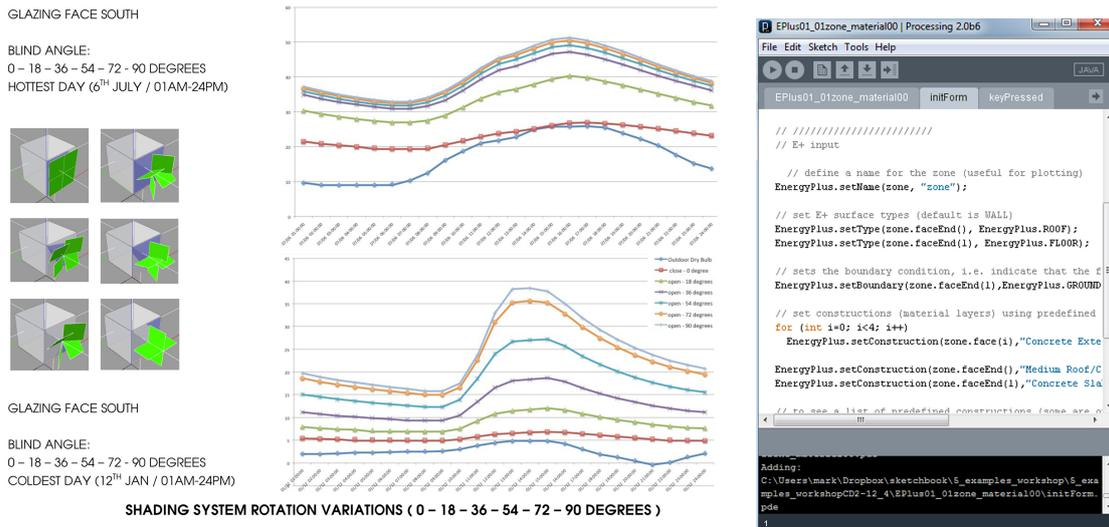
Figure 1: Final assignment: a parametric shading system adapting to different orientations. Example design and analysis produced by the students (Vinh Nhy Ly) (left). Example script within the Processing IDE, focused at EnergyPlus related functions (right).
