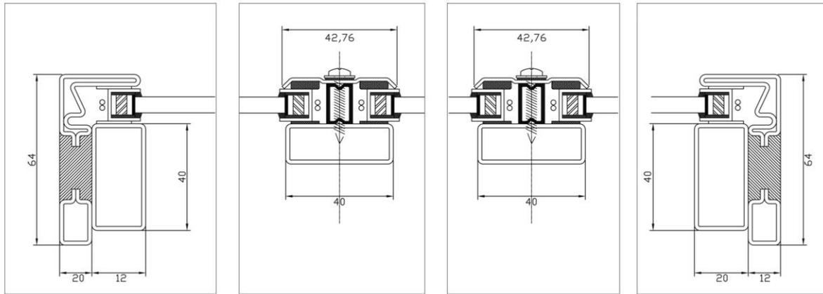
Figure 5: Design of the steel profile of the window. longitudinal section.
