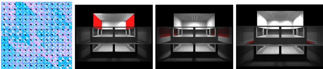
Figure 3: Filter optimization for an homogeneous filter (left), the black triangles represent the pattern and the rest of triangles, the associated mesh. Three different lighting intentions (from left to right: lateral upper walls, first floor walls and first floor) where designed to obtain the corresponding filters.
