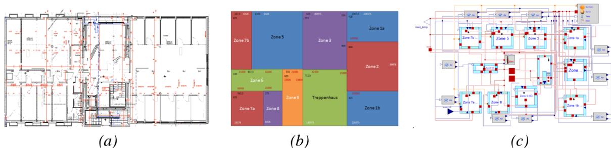
Figure 2: a) Floor plan of the first floor b) Zoning of the first floor in the model
