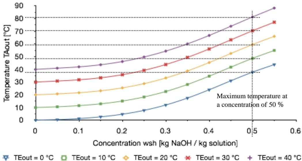
Figure. 2. Maximum output temperature in respect to sodium hydroxide concentration and solvent evaporation temperature.
