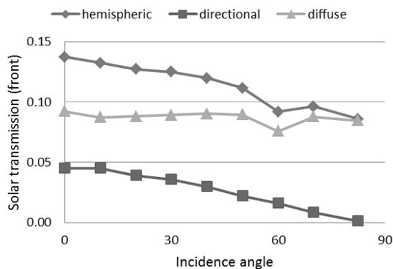
Figure 2: Hemispheric Front Solar Transmittance of Sc1
