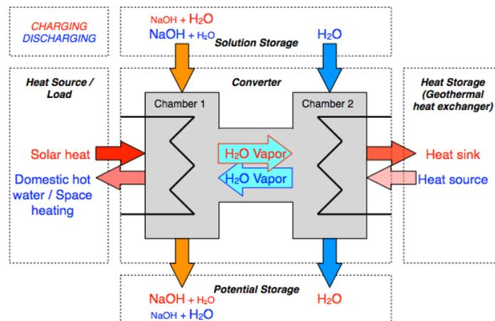
Figure 1. The concept of the closed sorption heat pump based heat storage.
