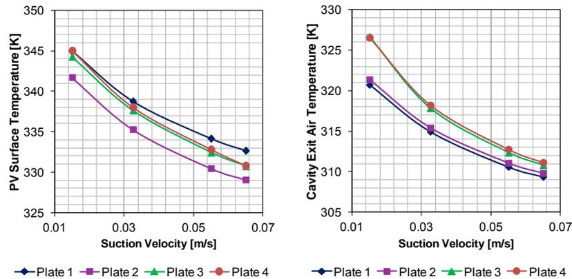
Figure 3: Comparison of PV surface temperature (left) and cavity exit air temperature (right) for plates 1 – 4 under different suction velocity
