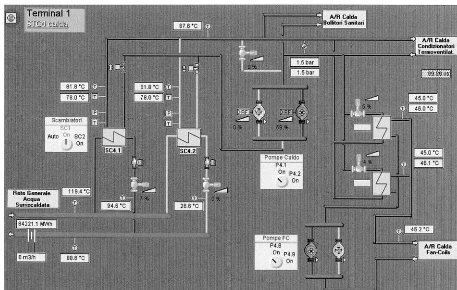
Figure 5: P&ID of a Heating Circuit in Terminal 1 of Mailand Malpensa Airport [12]
