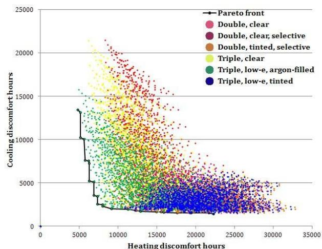
Figure 2: Building variants colored according to southern glazing type.
