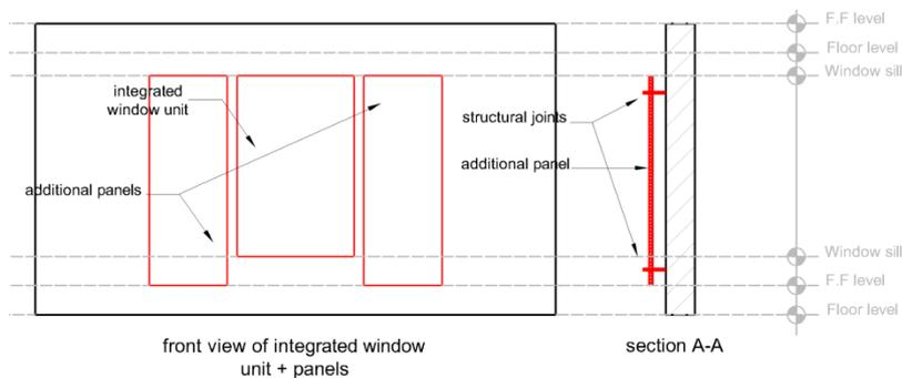
Figure 4:Window module unit with additional panels.
