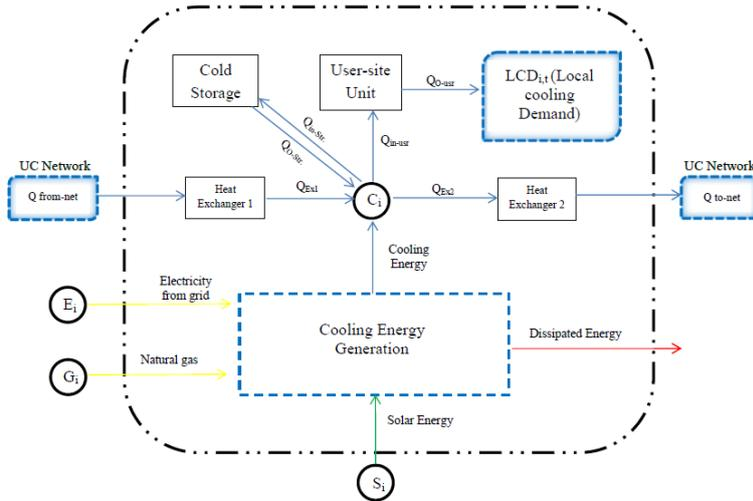
Fig. (3): Local Cooling Energy System (Superstructure) at site (i). Where : G<sub>i</sub> represents the local fuel (Gas) supply system, E<sub>i</sub> represents the local electricity supply grid, S<sub>i</sub> represent the solar energy resources and C<sub>i</sub> represents the local cooling supply piping system.
