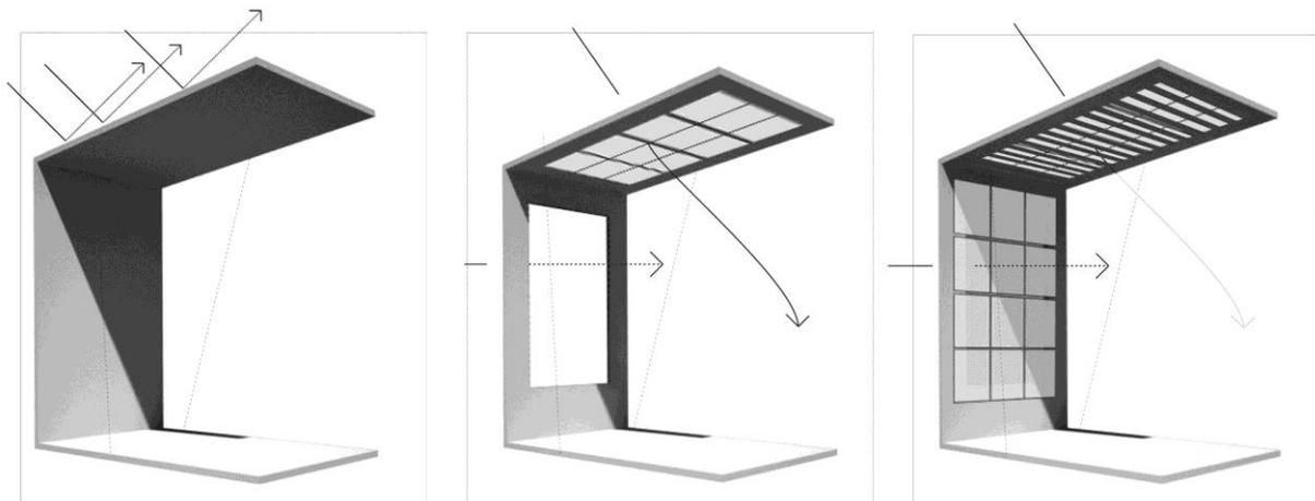
Figure 2: The three possible types of energy modules (from left to right): “full module” (with a reflective panel), “empty module” (the coloured light pass through) and “shielded module” (with slats that filter light).
