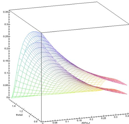
*Figure 4: Irradiance increase onto the collector plane, with respect to the sun elevation ( $\alpha_s$ ) and collector plane irradiance angle ( $\theta_2$ ) when taking the polarization effect into account (lower plane) resp. when neglecting it (upper plane). Over all, the effect lowers the irradiance enhancement by 1/5.*
