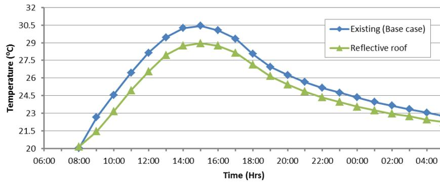
Figure 2. Hourly air temperatures observed in ENVI-met for reflective roofs in comparison with the existing (basecase) scenario
