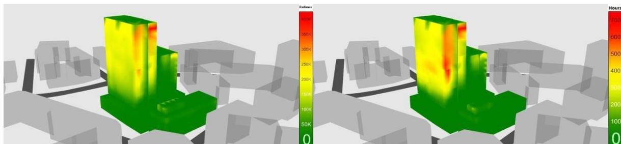
Figure 4: Left: Colour coded cumulative radiance on the assessed building envelope. Right: Hour count of luminance above threshold of  $10000 \text{ cd/m}^2$  displayed on the assessed building envelope
