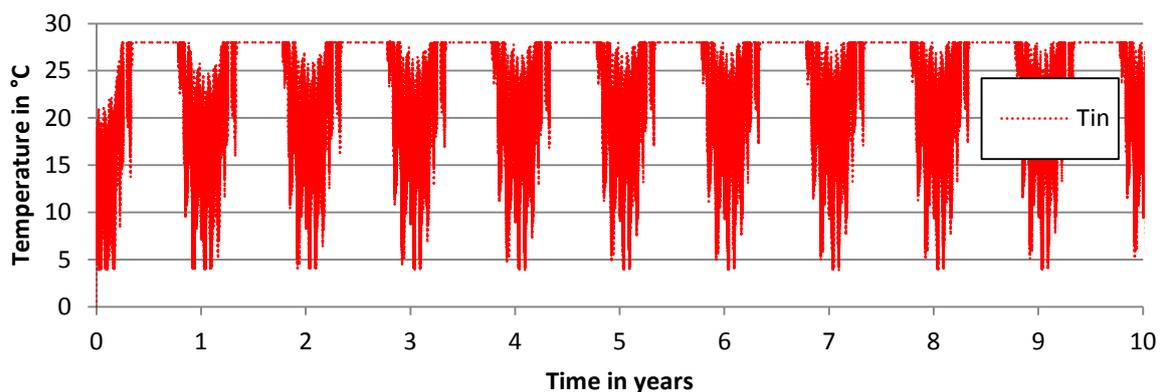
Figure 3: Input temperatures at the “Grünmatt” ground storage simulated for ten years with the TRNSBM model based on a maximal temperature range of 4..28°C. (Coloured graph only available in the digital version of the paper)
