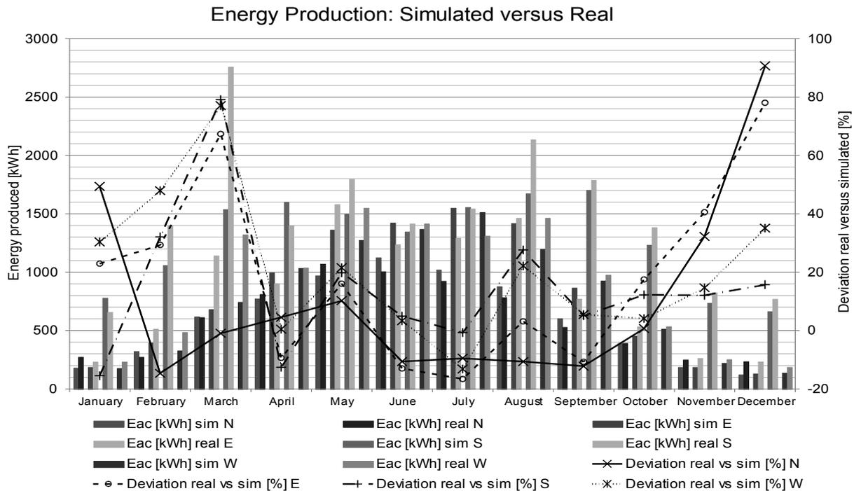
Figure 1: Simulated yield data versus real energy production with deviation (Real/Sim)
