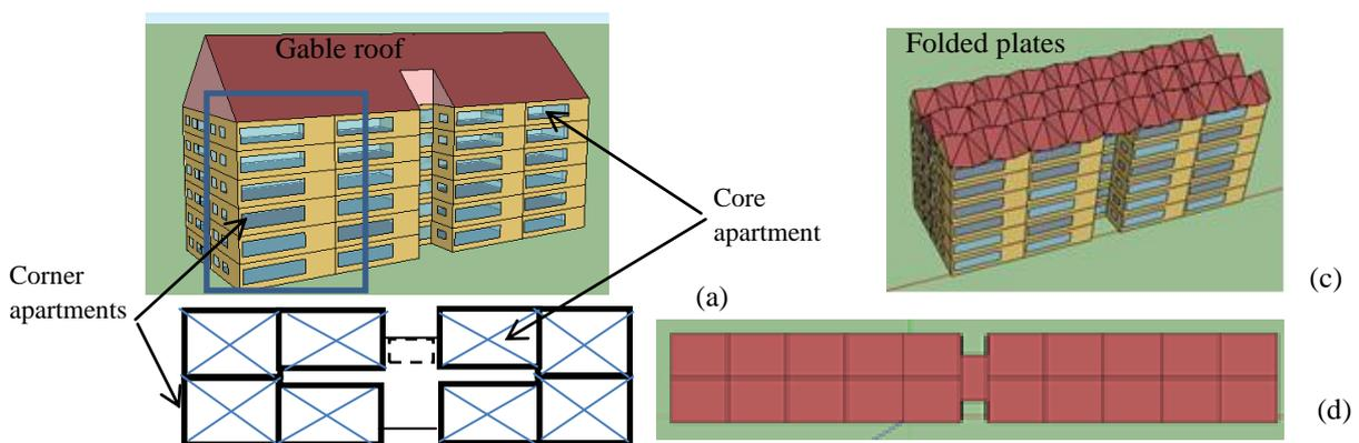
Figure 3 Apartment building: (a) view with gable roof, (b) Plan, (c) view with folded plate roof, (d) Maximum apartment buildings within an acre.
