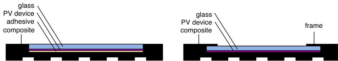
Fig.1. Standard lamination (left) and integrated process (right).
