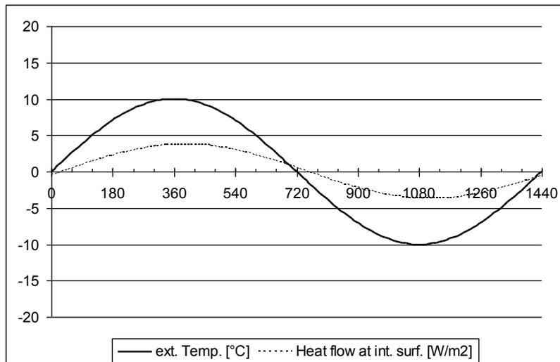
Figure 3 Thermal insulation panel: heat flow rate through the internal surface [ $\text{W/m}^2$ ] (dotted thin line) and outdoor temperature in  $^{\circ}\text{C}$  (continuous thick line) over the period of one day (x-axis).
