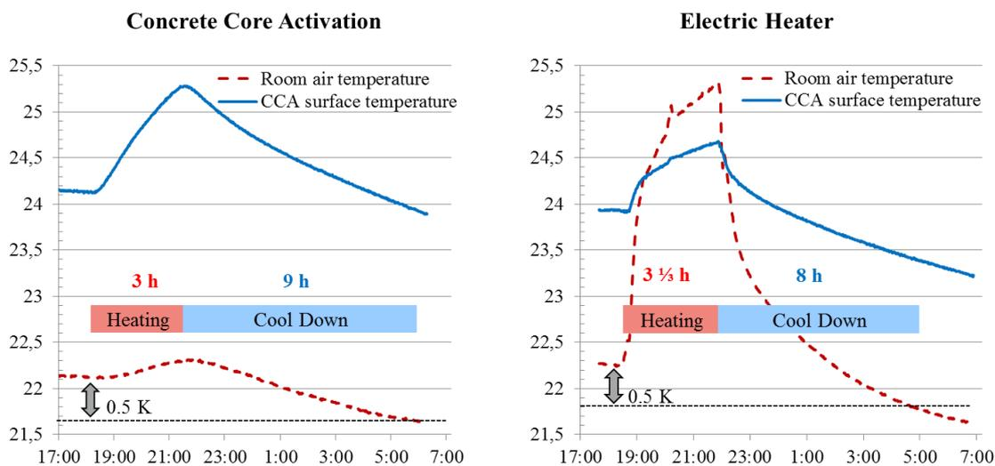
Figure 2: Comparison of measured overheating and cool down phases
