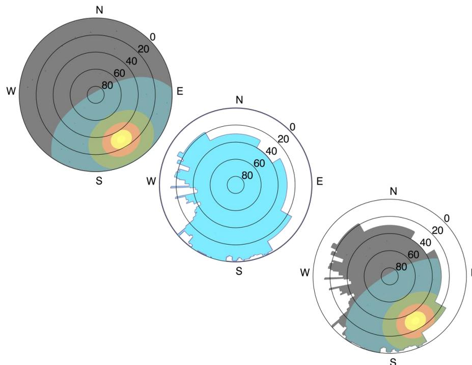
*Figure 1: Illustration of the shadowing analysis for the diffuse irradiation for a specific point in time: radiation distribution (left), horizon (center) and un-shadowed part of the radiation distribution.*
