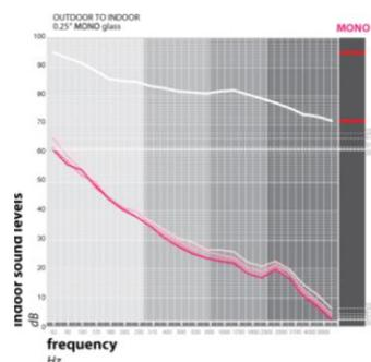
Fig. 5: Simulated sealed double-skin façade composed of monolithic glass under ISO 717.
