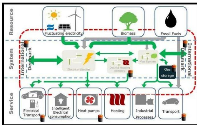
*Figure 2: Modelling framework architecture.*
