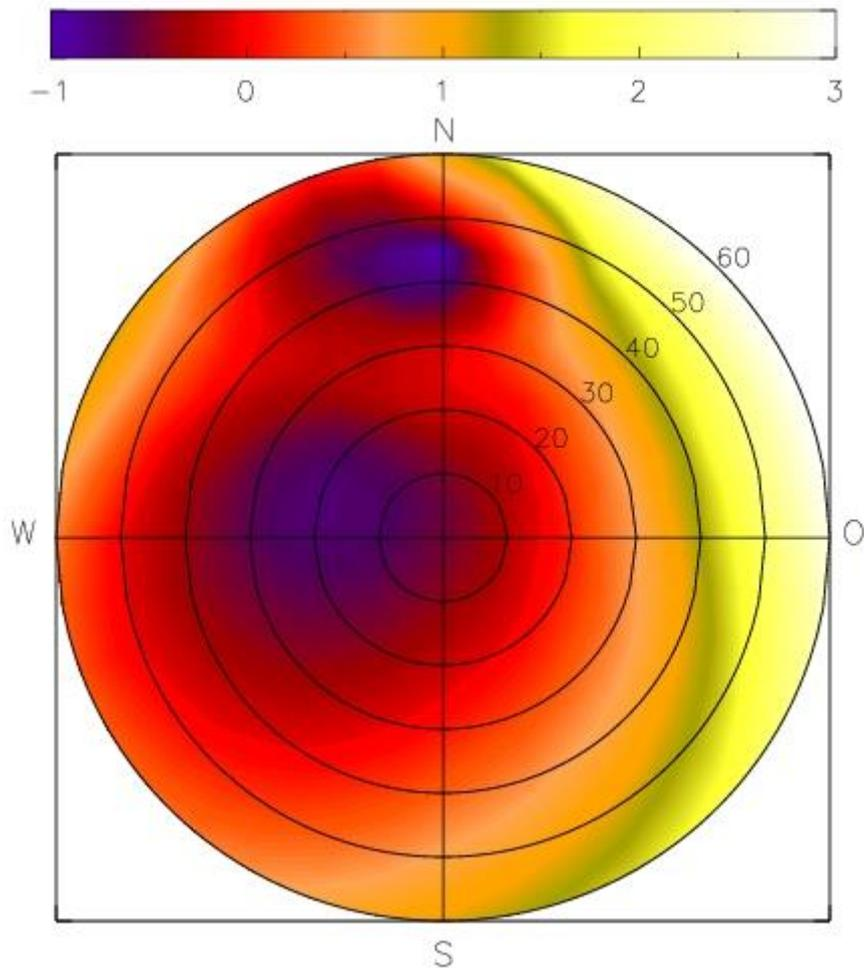
Figure 3: Distribution of the mean relative error (MRE) in % depending on the orientation and inclination of the roof plane for 120 months the validation period 2002-2011.
