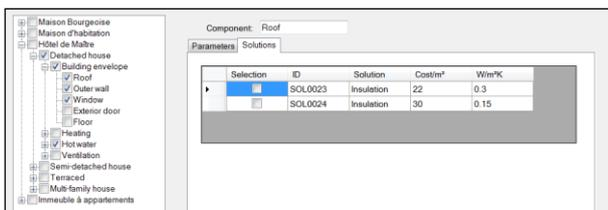
The picture in the left shows an example of a cell in the TCS matrix in the current version of the tool, which contains different solutions applicable to roofs in buildings in the scope of the study. The final number of solutions will be increased along with the study,
