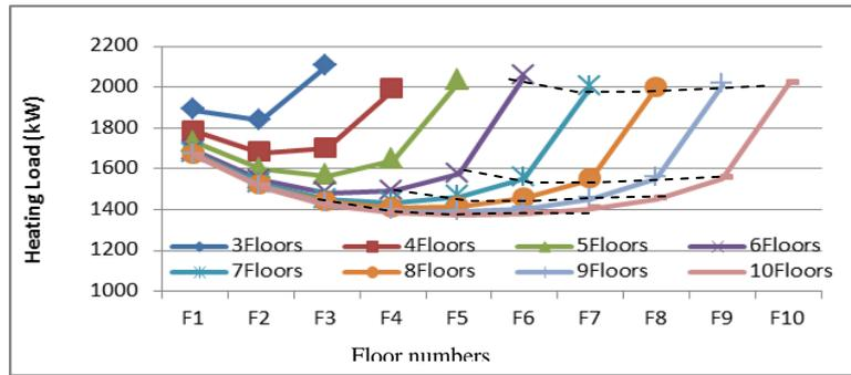
Figure 4, Average heating load for each floor in apartment buildings.
