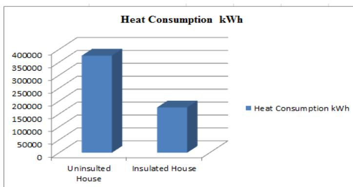
Figure 3 Heat consumption results calculated by software tool for un-insulated and insulated prototype building
