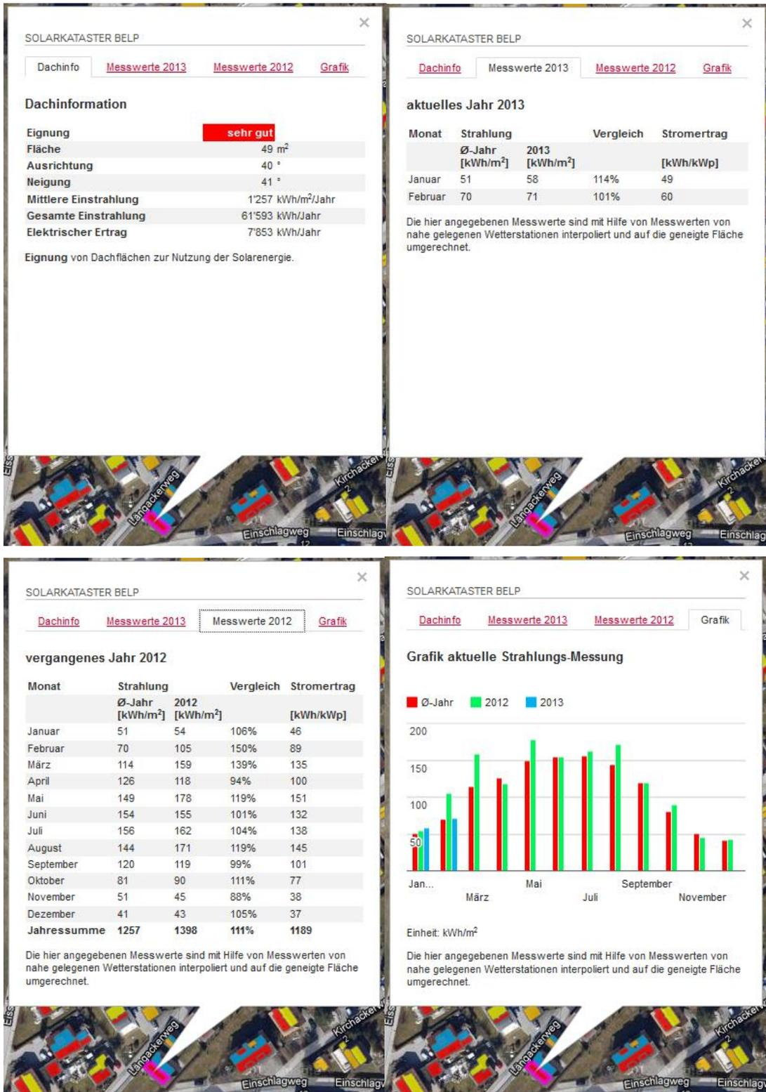
Figure 4: Screenshots from the website <http://solarkataster.meteotest.ch/belp> which shows the monthly irradiation data and the estimated production.
