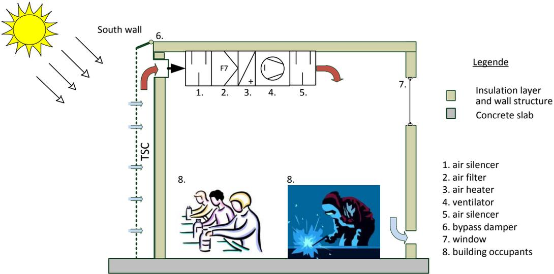
Figure 2: Schematics of the generic TSC system including ventilation system but without air-to-air heat recovery) (Illustration 8: © office.com)
