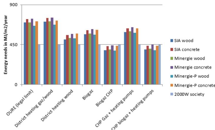
Figure 5: constructive modes and energy supply comparison. QuaD project, CREM
