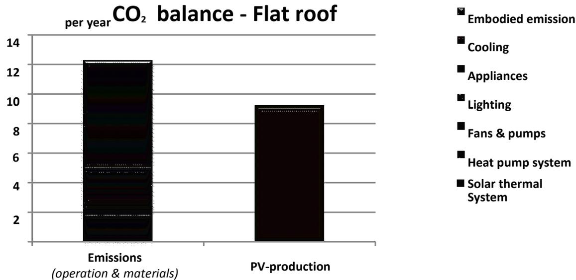
Figure 4 CO<sub>2</sub> balance between emissions from energy used for operation & embodied emissions from materials, and PV production with roof mounted PV.
