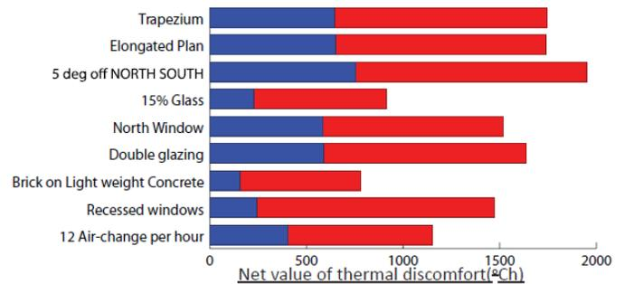
Graph 1: Graph illustrating the net values of thermal discomfort for the best performing passive design parameters highlighted in Table 3.
