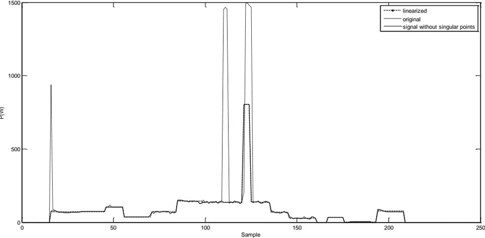
Figure 5: Active Power: measurements, corrected, linearized
