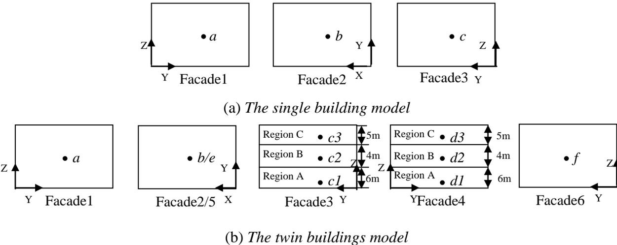
Figure 4: Positions of nodes extracted from each facade
