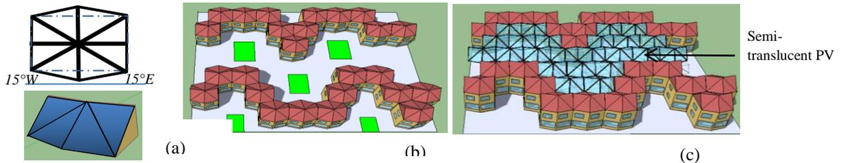
Figure 2 Hexagonal units; (a) roof design, (b) Configuration of multiplex, (c) multiplex with external structure
