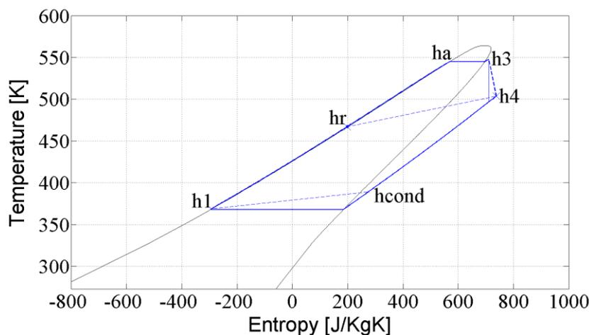
Figure 2: T-S diagram of the organic Rankine cycle with regenerator.
