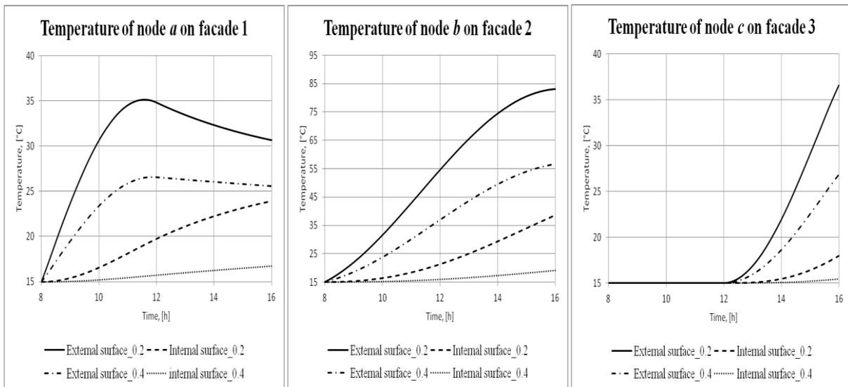
Figure 6: Comparison of temperature for different wall thicknesses
