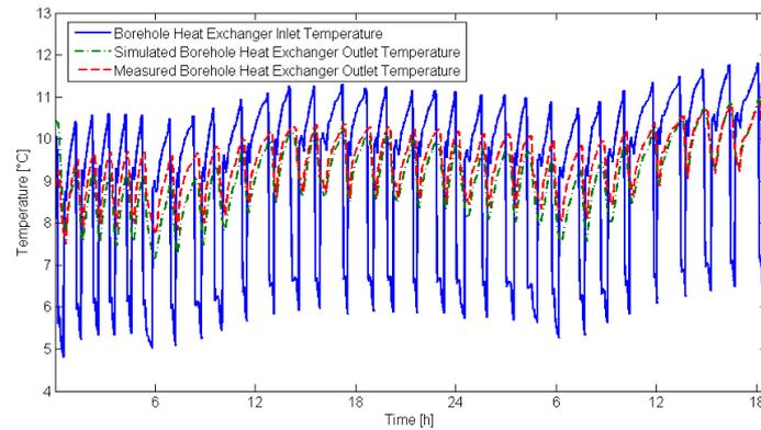
Figure 6: Borehole heat exchanger inlet and outlet temperatures
