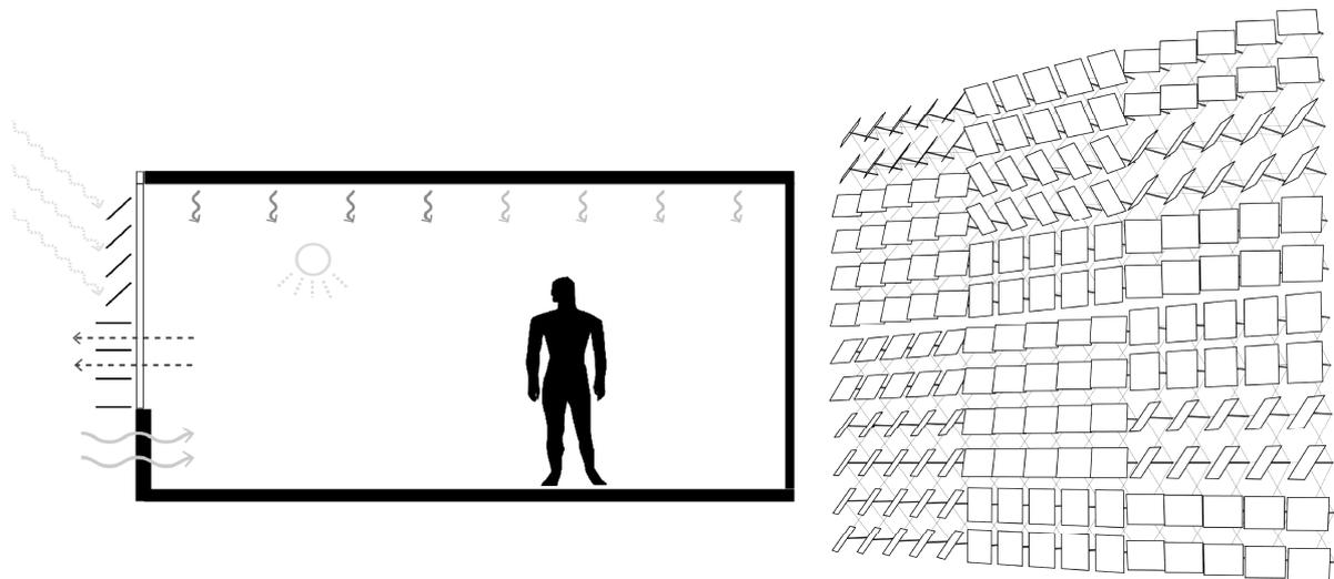
*Figure 1: Environmental factors that can be influenced by adaptive solar façade systems include solar insolation, views, heating/cooling loads and artificial lighting loads (left). Adaptive solar façade elements in various orientations (right).*
