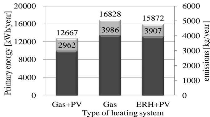
Figure 4: Primary energy consumption and CO<sub>2</sub> emissions for different heating systems.
