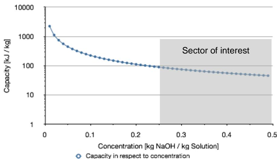
Figure. 3. Shows the reduction of the capacity gain in respect to the sodium hydroxide concentration in the solution.
