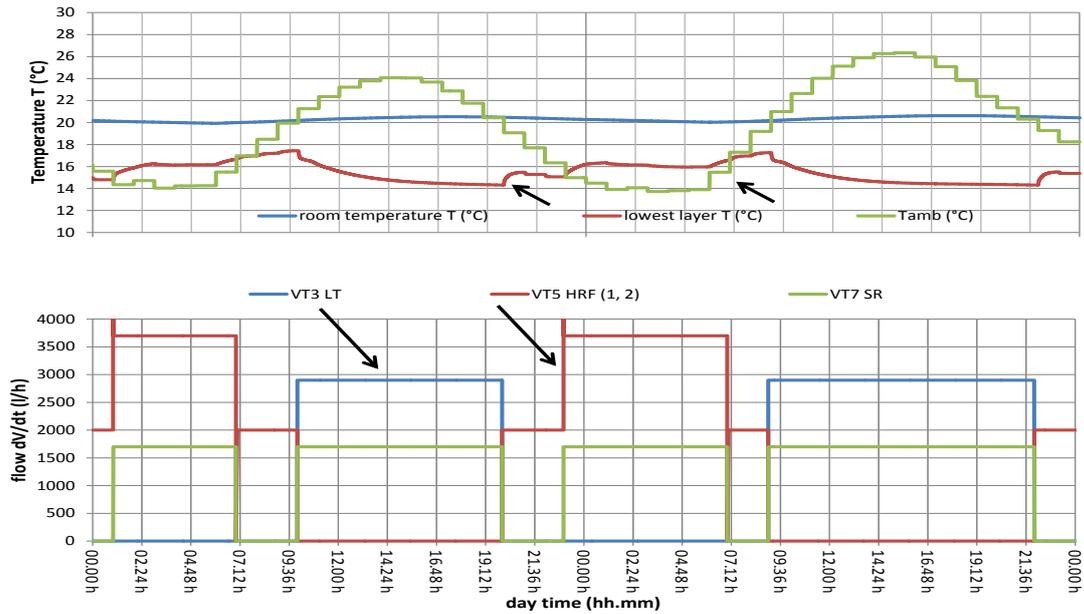
Figure 4: Temperature of the server room, the lowest layer in the cold storage tank and the ambient air in function of time over two days (above). The building in the template of Figure 3 represents the server room (SR). The ambient temperature has a hourly resolution and is staircase-shaped. The lower graph of the Figure shows the fluid flow in the pumps VT3 LT, VT7 SR and VT5 HRF (1, 2) of the template in Figure 3.
