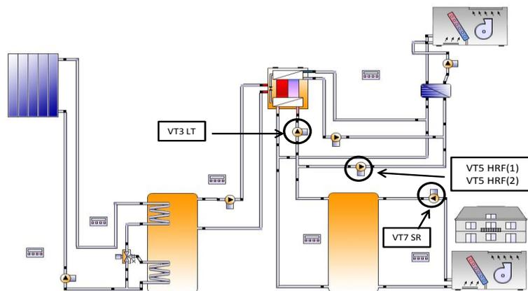
Figure 3: Schematic of the graphical user interface in the POLYSUN-Software of the solar thermal driven 8kW adsorption cooling machine ACS08 of SORTECH AG. In the simulation the volume flows of VT3 LT, VT5 HRF(1) and VT5 HRF(2) will be realised by two pumps running with a programmable controller.
