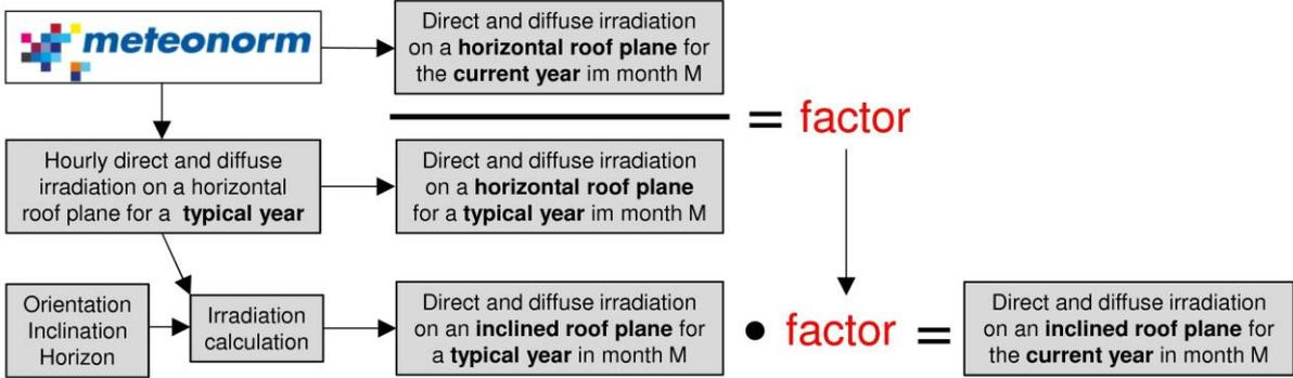
Figure 2: Illustration of the method to estimate the monthly irradiation values for the current year based on measured irradiation data on a horizontal plane.
