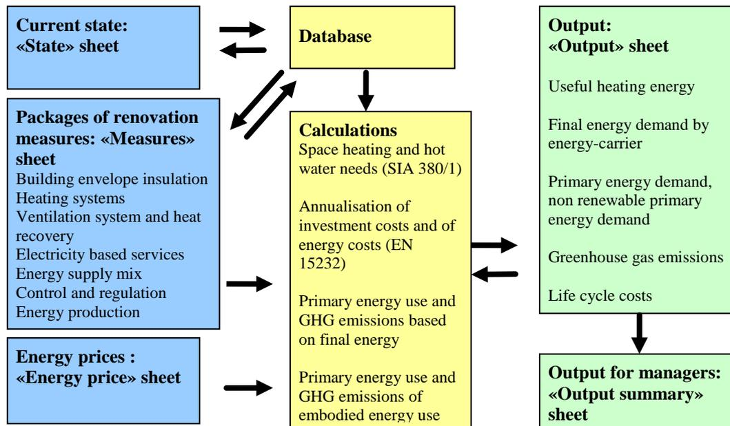
Figure 1: Schematic structure of the INSPIRE tool
