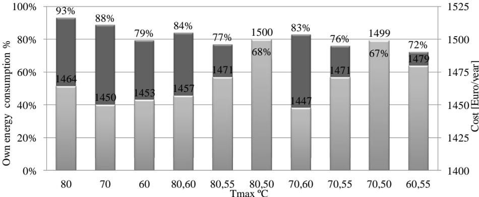
Figure 1: The black columns are total energy consumption from PV panels and the gray columns are energy costs balance with different values of Tmax.
