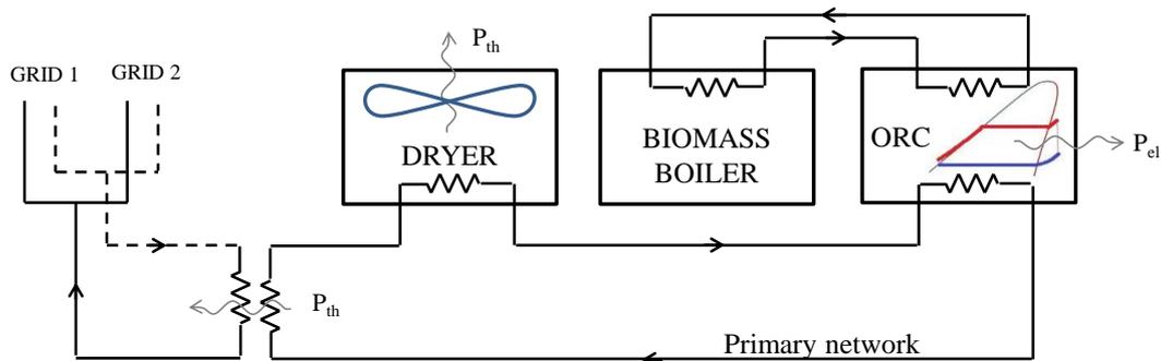
Figure 1: Schematic diagram of the power plant components.
