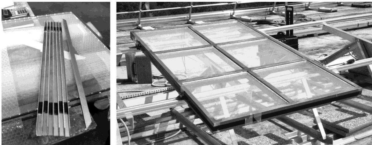
Figure 6: Metal edges for the LSC plates (left) and complete PV panel (right).
