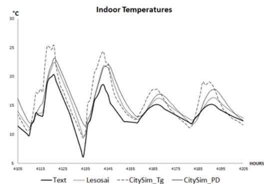
Figure 2: Inter-model comparison – Effect of penetration Depth.
