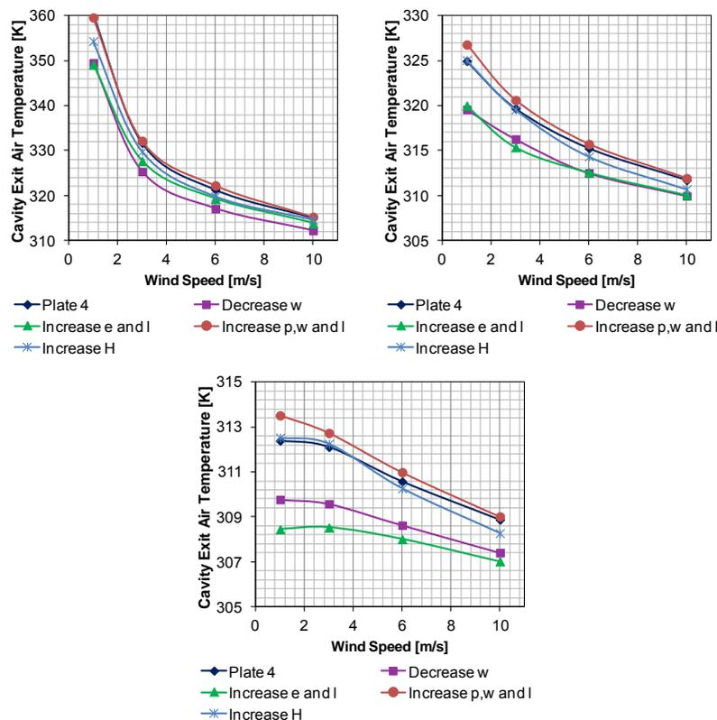
Figure 4: Comparison of cavity exit air temperature for different geometry shapes under different suction velocity: 0.01 m/s (left), 0.03 m/s (middle) and 0.06 m/s (right)
