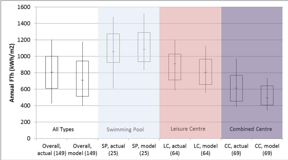
Figure 2: A comparison of actual Fossil-Thermal (FTh) energy use against modelled energy use, showing median, 10<sup>th</sup>, 25<sup>th</sup>, 75<sup>th</sup> and 90<sup>th</sup> percentiles, split by building type.
