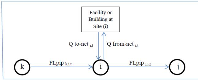
Fig. (2): energy-flow structure of the UC network at site (i).
