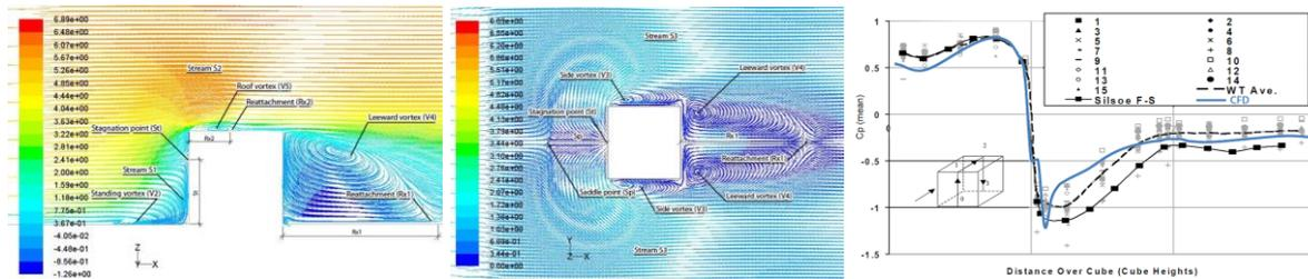
Figure 2 Left (a), middle (b) vertical and horizontal stream wise velocity path lines. Right (c) Pressure coefficients along the centreline of the cube.
