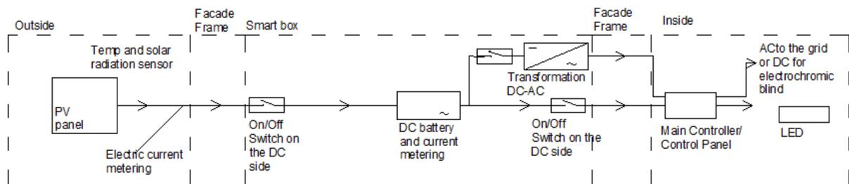
Figure 7: PID of PV window module
