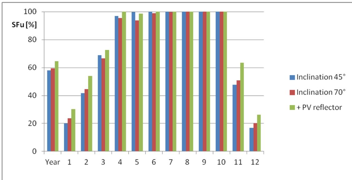
Figure 5: Solar fraction for the Minergie-P-ECO building with a specific consumption of 15 kWh/m<sup>2</sup> of energy reference area. The building is exactly southwards oriented. The thermal field has once been simulated with 45° inclination, than with an inclination of 70°, and finally with 70° inclination and a PV field below the thermal field with 11° of inclination.
