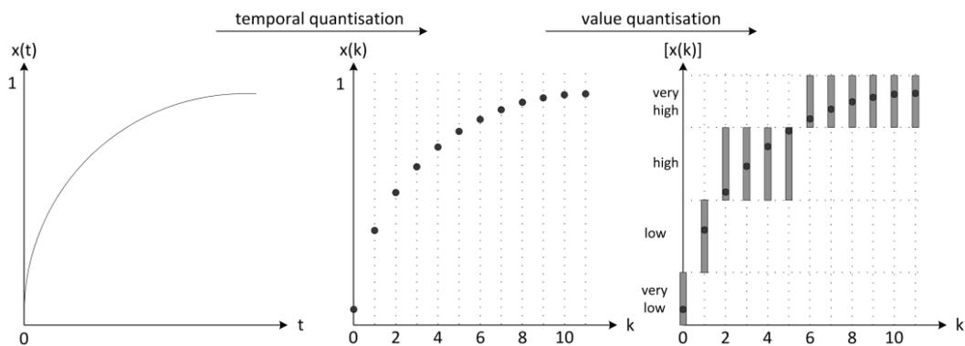
Figure 3: Signal quantisation, based on [3]
