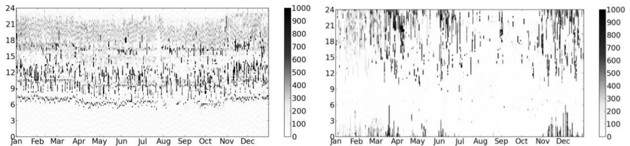
Figure 7: Carpet plot of electric load profiles for different households. Some have very regular daily patterns (left: AP02), especially the loads during night and day can differ significantly (right: AP03).
