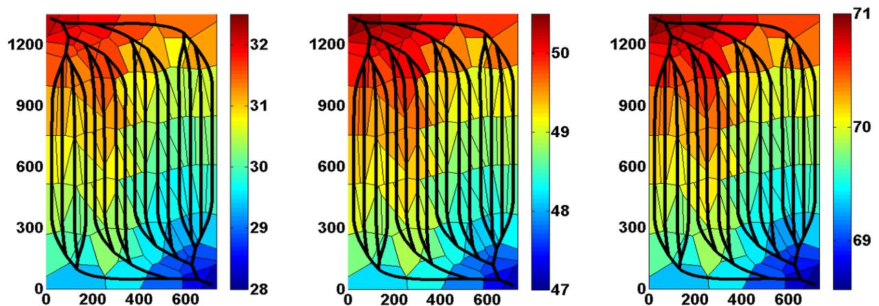
Figure 1: Temperature fields in the exchanger for  $T_{inlet} = 28.1^\circ\text{C}$  ;  $T_{inlet}=48.5^\circ\text{C}$  and  $T_{inlet}=68.2^\circ\text{C}$
