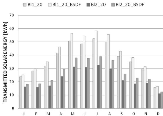
Figure 6: Monthly transmitted solar energy through window for B11\_20 and B12\_20.
