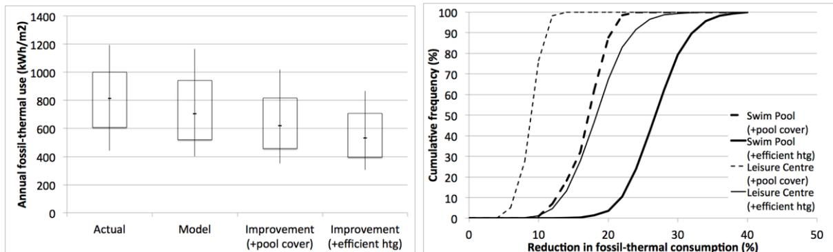
Figure 3: Impact of improvements on FTh consumption across all buildings (left); the range of % reduction in FTh consumption in an example swimming pool and leisure centre (right).
