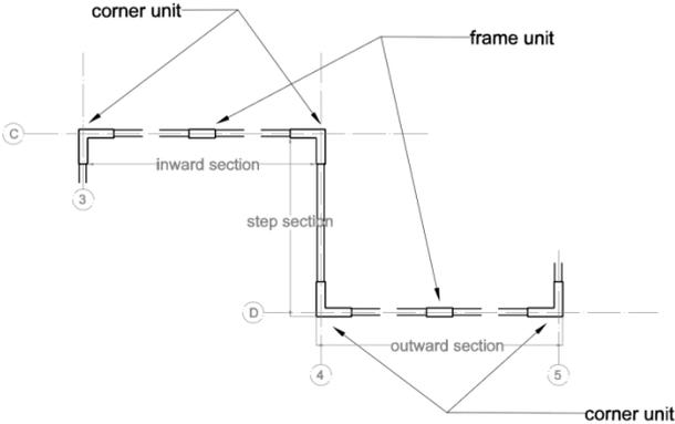
Figure 2: System level of the design. Different types of modules.
