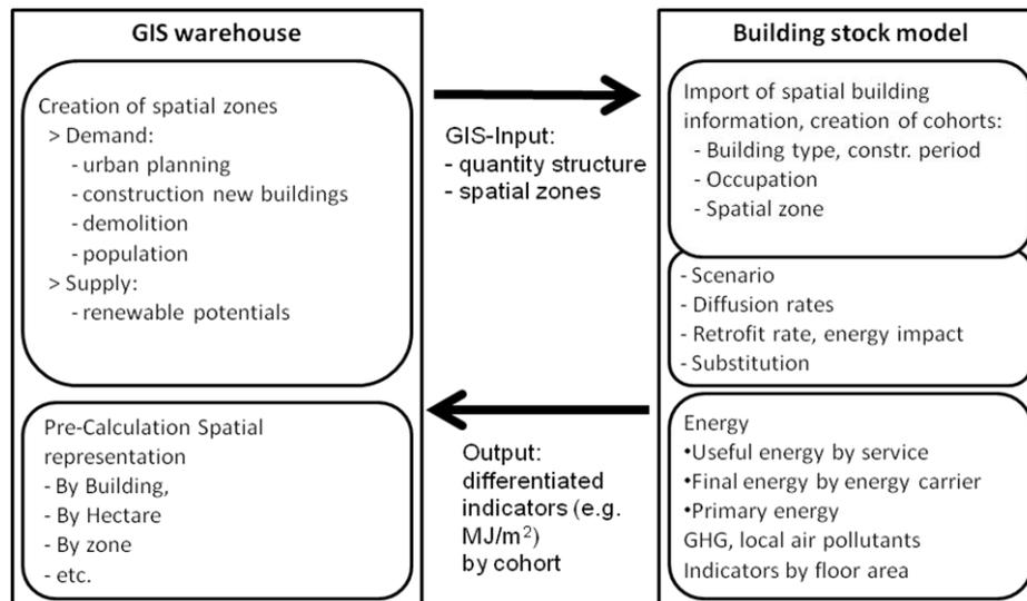
Figure 1: Interaction of the building stock model (BSM) with geo-referenced data and the GIS environment
