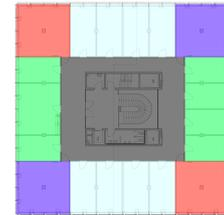
Figure 3: Exemplary floor plan with thermal zoning.
