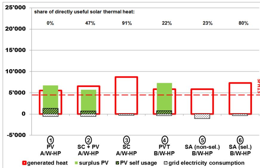
Figure 4 Results of the system comparison for the building SFH15
