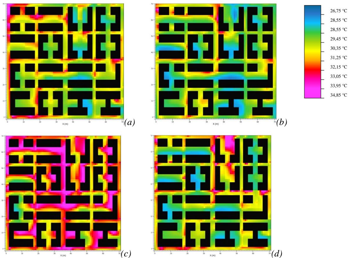
Figure 8. ENVI-met results urban air temperature, horizontal profile at 3m height in August 2<sup>nd</sup>, 3pm in four scenarios: (a) real, (b) RIE, (c) impervious surfaces, (d) cool surfaces.
