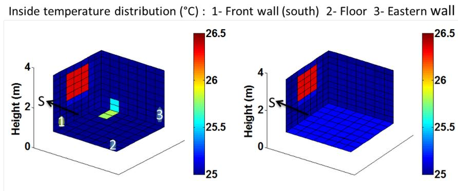
Figure 3: a/ with sun patch (M2) b/ incoming radiation projected on the floor (M1)
