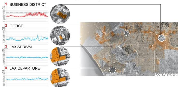
*Fig. 6: Outdoor sound levels obtained from field-measurements to compose a mapping tool indicating façade parameters necessary to respond to indicated outdoor sound conditions.*
