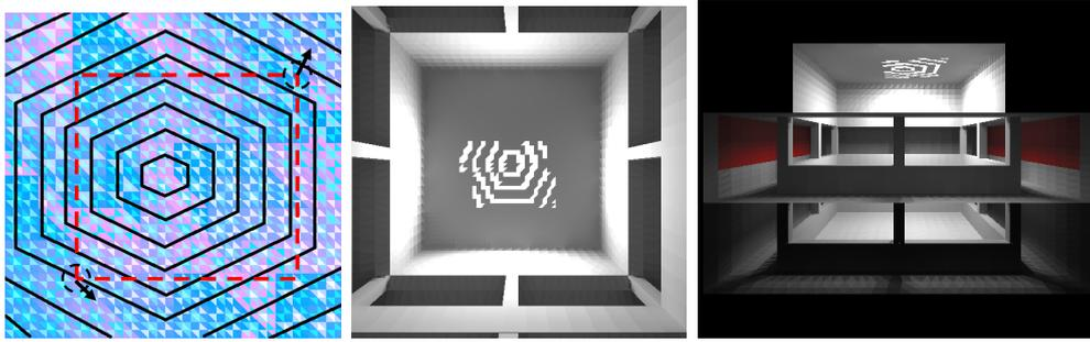
Figure 4: Filter optimization using an hexagonal pattern filter (left) and the resulted filter (middle) for given lighting intention at the lateral (in red) walls (right).
