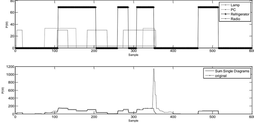
Figure 6: load curve: single appliances (above), total load (below)
