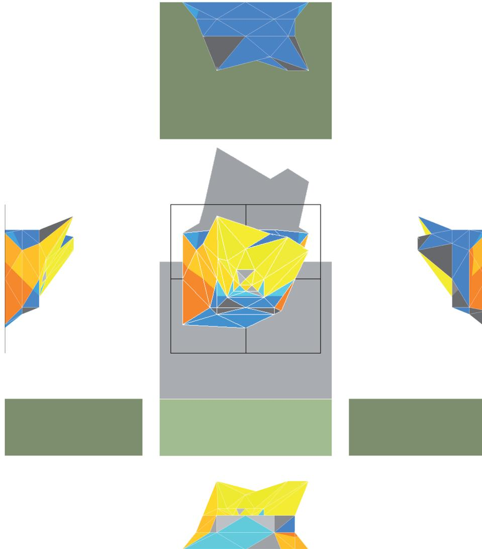
Figure 5: Best individual of the last generation in the optimization with a large and tall obstacle. Top view in the centre, East, South, West and North façades respectively on the right, bottom, left and top.
