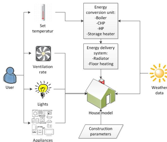
Figure 1: Set-up of a house model
