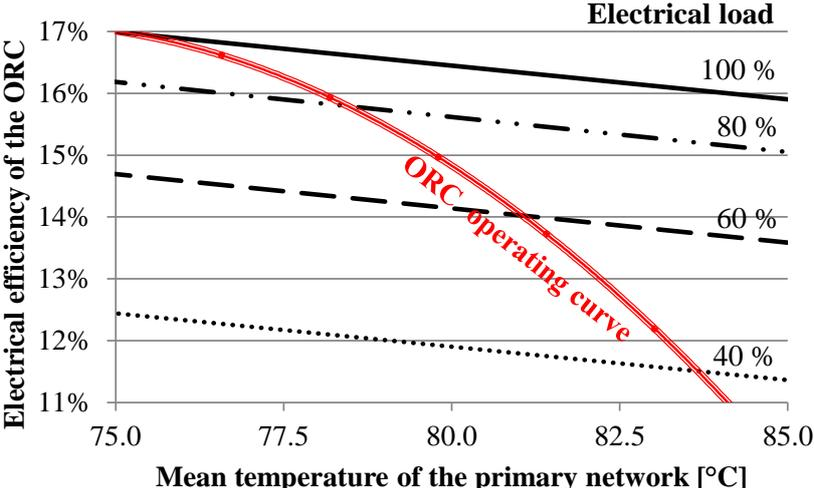
Figure 4: Electric power trend as a function of the mean temperature of the primary network
