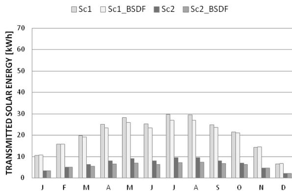
Figure 4: Monthly transmitted solar energy through window for Sc1 and Sc2.
