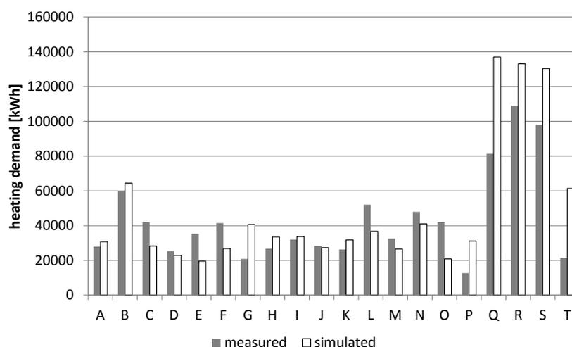
Figure 1. Comparison between measured and simulated heating demand of buildings
