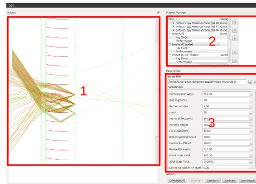
Figure 3: Graphical User Interface. Area 1 shows the output, in this case ray tracing. Area 2 shows the project list. Area 3 the parameters listed in the script.
