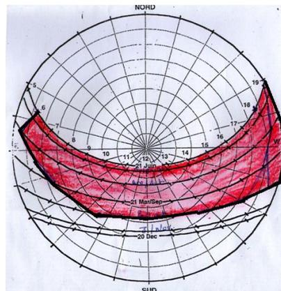
Figure 3: Polar diagram of Biskra, presentation of the superheated zone
