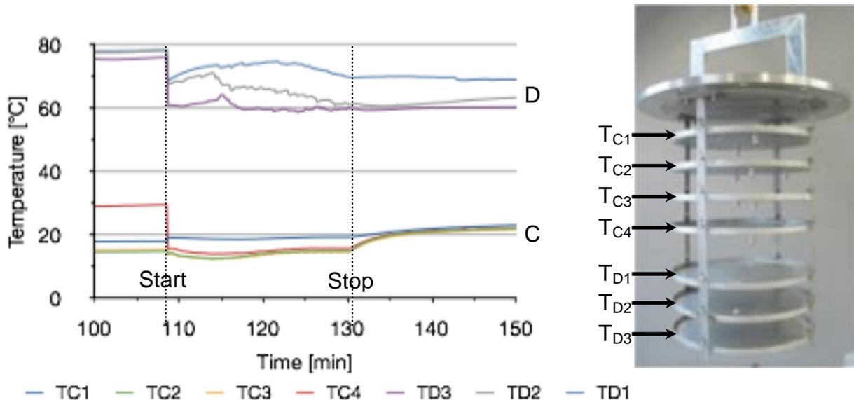
Fig. 5. Diagram of the regenerating process. The temperatures of the desorber as well as the condenser plates are shown.
