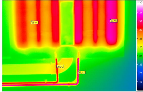
Figure 7: Thermal image of radiant panel in operation on an average winter day with  $\Delta T(\text{Water}) = 2.3^\circ \text{C}$ . Emissivity value  $\varepsilon = 0.9$  assumed for all surfaces.
