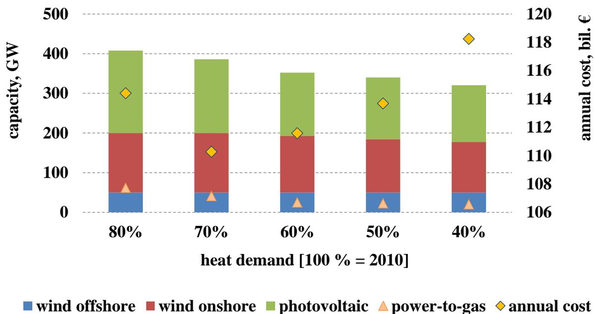
Figure 2: Installed capacity of different technologies and the total system cost depending on the amount of energy saving retrofit measures
