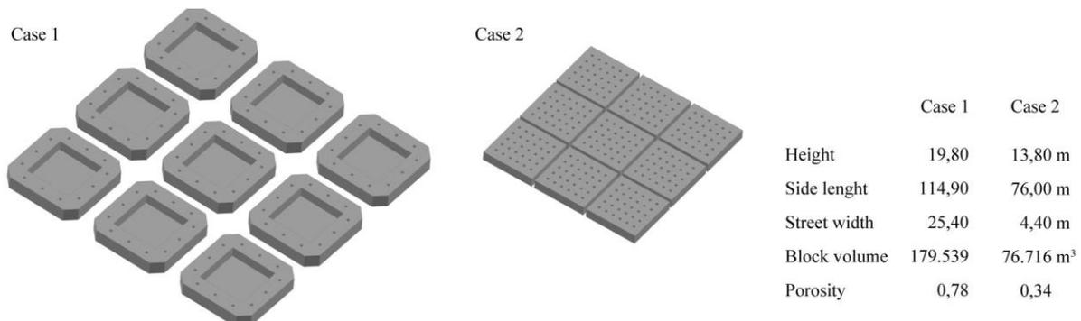
Figure 3: Typological models of the Eixample (left) and Barri Gotic samples (right)
