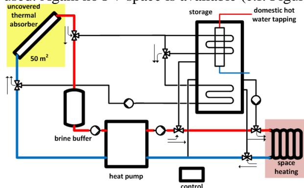
Figure 3 System and hydraulic scheme of system 5 and 6
