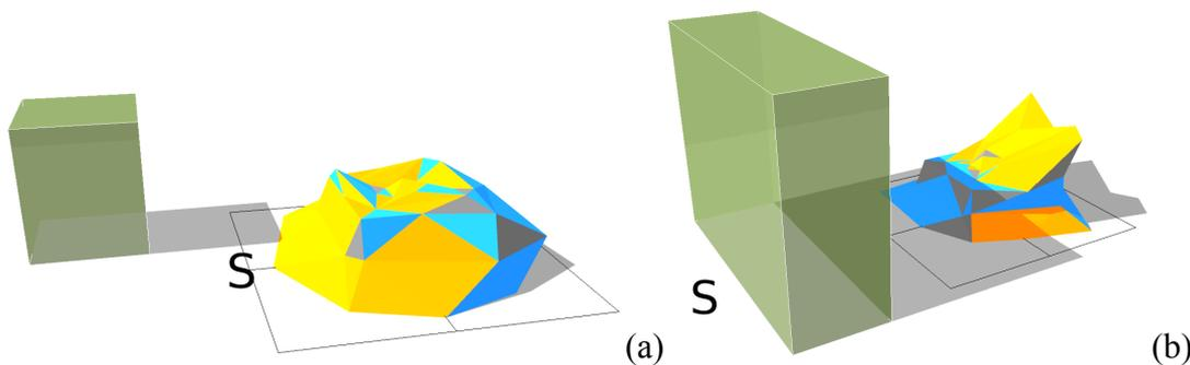
Figure 6: Perspective view of the optimized envelopes in the presence of a small (a) and a large and tall (b) obstacles.
