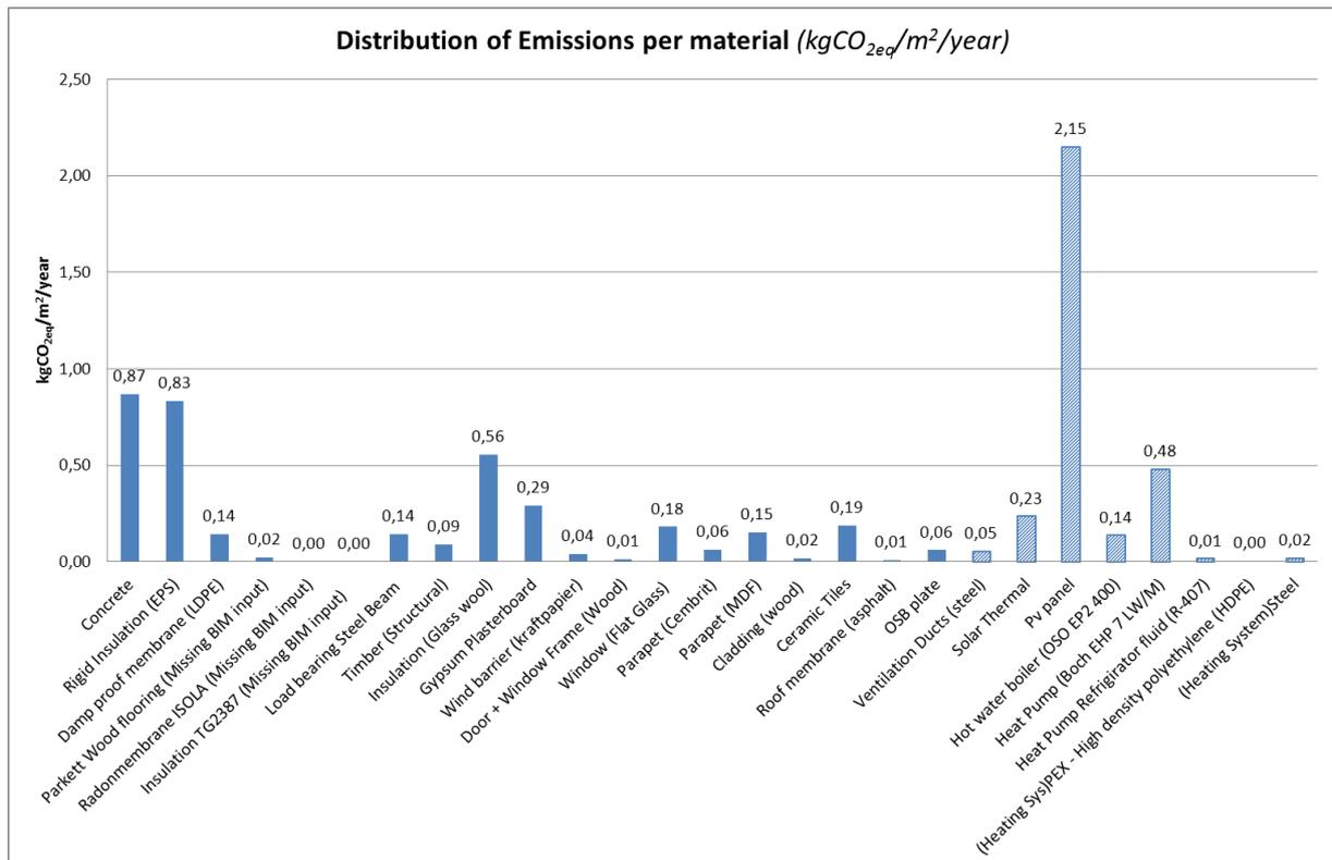
Figure 3 Distribution of carbon dioxide emissions (kgCO<sub>2eq</sub> per m<sup>2</sup> per year) from material and technical inputs.
