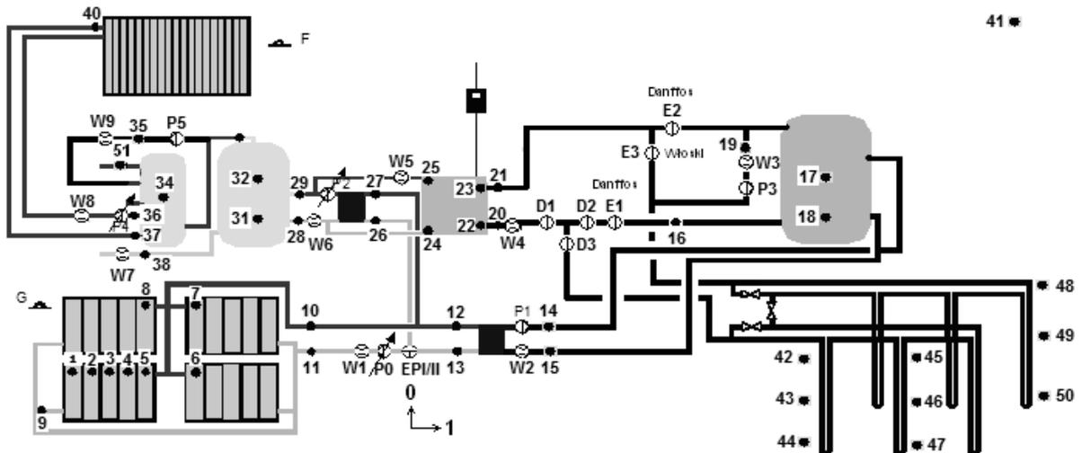
Figure 4. The principles of the modernized hybrid system control in schematic layout; D - hand operated valves, E - electric valves EP - three way valve, P - circulation pumps.
