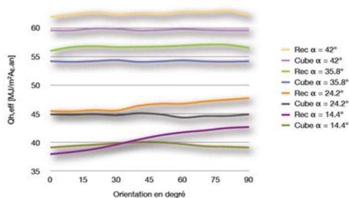
Figure 3: Energy-orientation correlation. Métamorphose project, Lausanne. The orientation of the buildings compared to a north-south axis implies a variation of the energy needs. The different colors represent the solar mask angle
