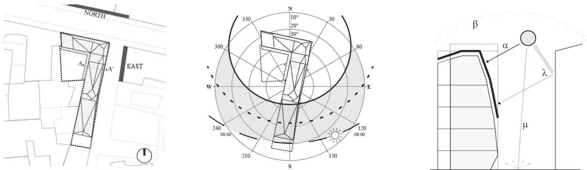
Figure 2. From the left side: site plan with the elevation of the analysed nearby buildings, the orientation of the building with respect to the sun path and section A-A' with different solar radiation components (sun ( $\alpha$ ), sky ( $\beta$ ), surroundings reflections ( $\lambda$ ), ground reflections ( $\mu$ )).
