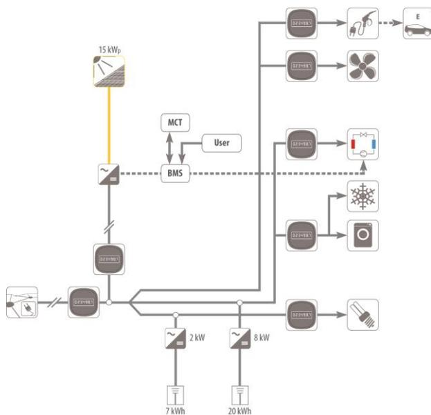
Figure 3: Electricity supply, -storage and -distribution and electricity meter concept
