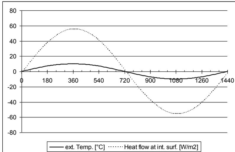
Figure 2 Glass pane: heat flow rate through the internal surface [ $\text{W/m}^2$ ] (dotted thin line) and outdoor temperature in  $^{\circ}\text{C}$  (continuous thick line) over the period of one day (x-axis).
