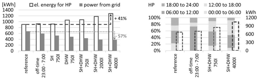
Figure 6: Due to changes in the control strategy the electric energy demand of the heat pump increases by 40%, because the heat pump is operated in unfavourable conditions (high supply temperatures) more often. Because the additional consumption is covered by PV the net electricity demand from the grid is reduced by nearly 60%.
