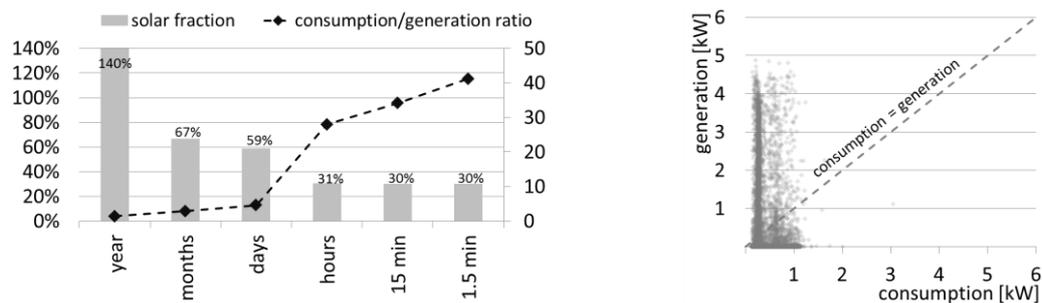
Figure 3: Solar fraction for the demo- building, relating to different time periods and equivalent ratio of consumption and generation (left) correlation plot of generation and consumption (right).
