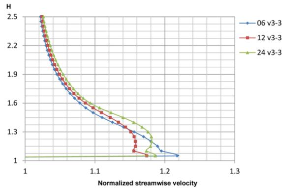
Figure 3 Comparison between the maximum recorded velocities at location v3-3 for the 3 heights
