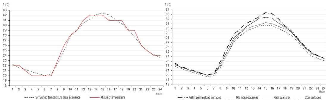
Figure 7. Measured (red line) and simulated hourly temperatures (dashed line) on August 2 2012(left). Hourly temperatures simulation on August 2 2012 for four cases scenarios (right).
