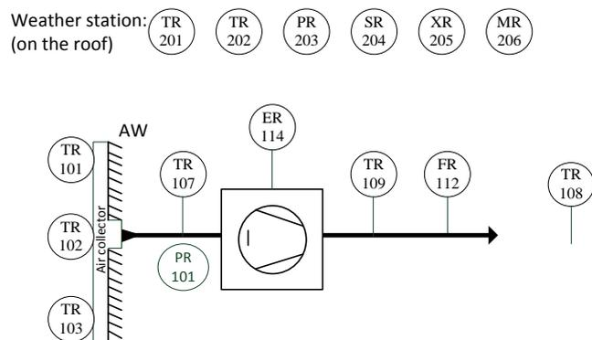
Figure 3: Schematics of the energy metering concept for the TSC system in Lucerne.
