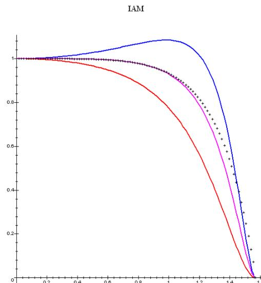
Figure 3: Angle dependence of the transmission of the transversal (upper solid line) and the longitudinal (lower solid line) polarization axis, as well as for unpolarized light (intermediate solid line). The dotted line is the IAM (incidence angle modifier) according to Ambrosetti, adjusted at 50° to the Fresnel equation.
