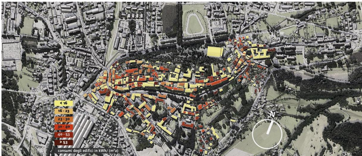
Figure 1: total energy consumption in KW/year per cubic meter of each building.
