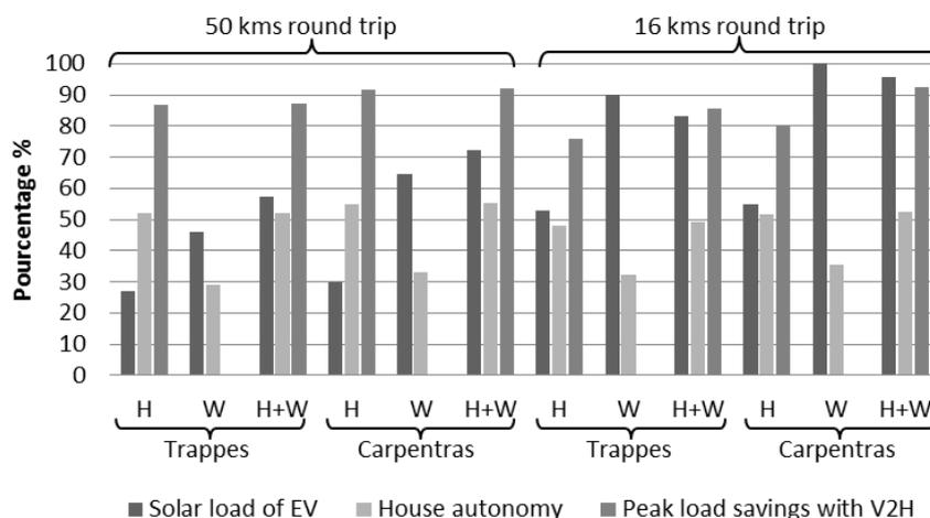
Figure 3: Solar load of EV, Building autonomy and Peak load savings with V2H for 3 plug-in modes – H (Home), W (Work) and H+W (Home & Work), 2 climates, 2 commuting distances
