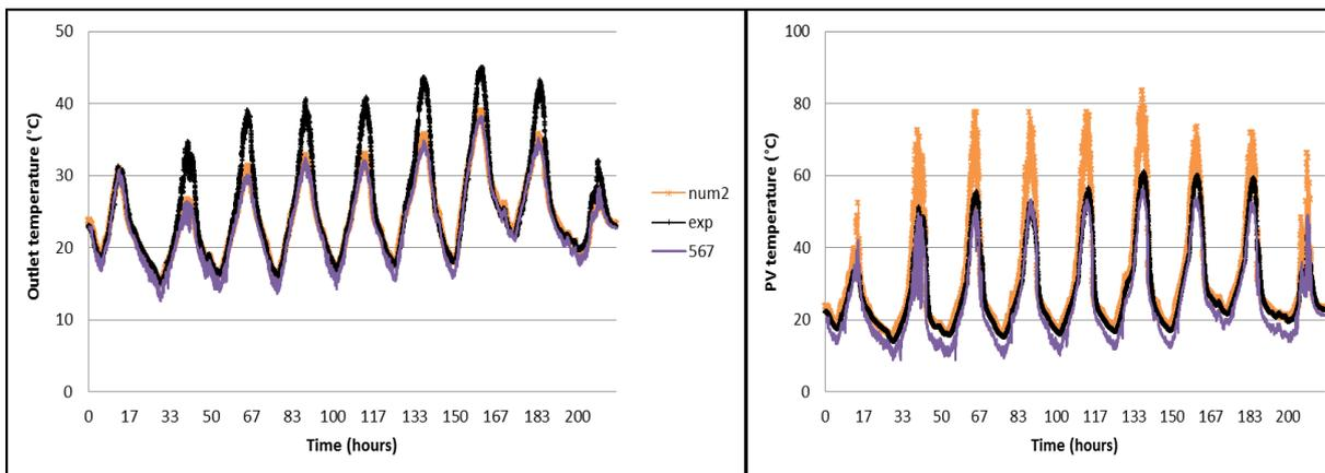
Figure 4 : evolution of outlet fluid temperature and PV cell temperature during 9 consecutive days in June (summer). Data series “num2” and “567” refer to the new and existing model.
