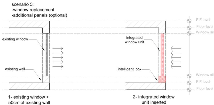
Figure 3:Section view of replacement of the window module unit.
