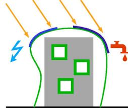
Figure 1: Solar Shell concept. External envelope's role is to produce heat and power.
