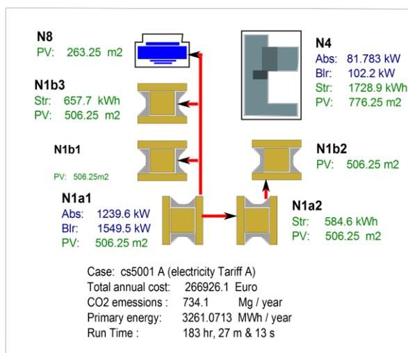
Figure (5): optimized cooling system obtained for Case study 2 for: Tariff A.
