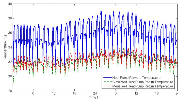
Figure 4: Heat pump forward and return temperatures
