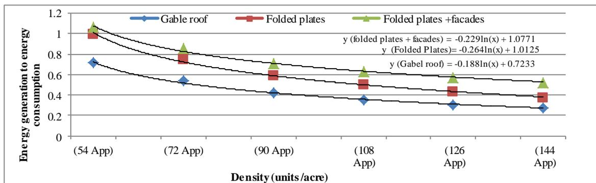
Figure 6, Energy balance vs density for different designs
