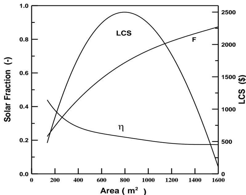
Figure 2: Variation of system parameters with collector area
