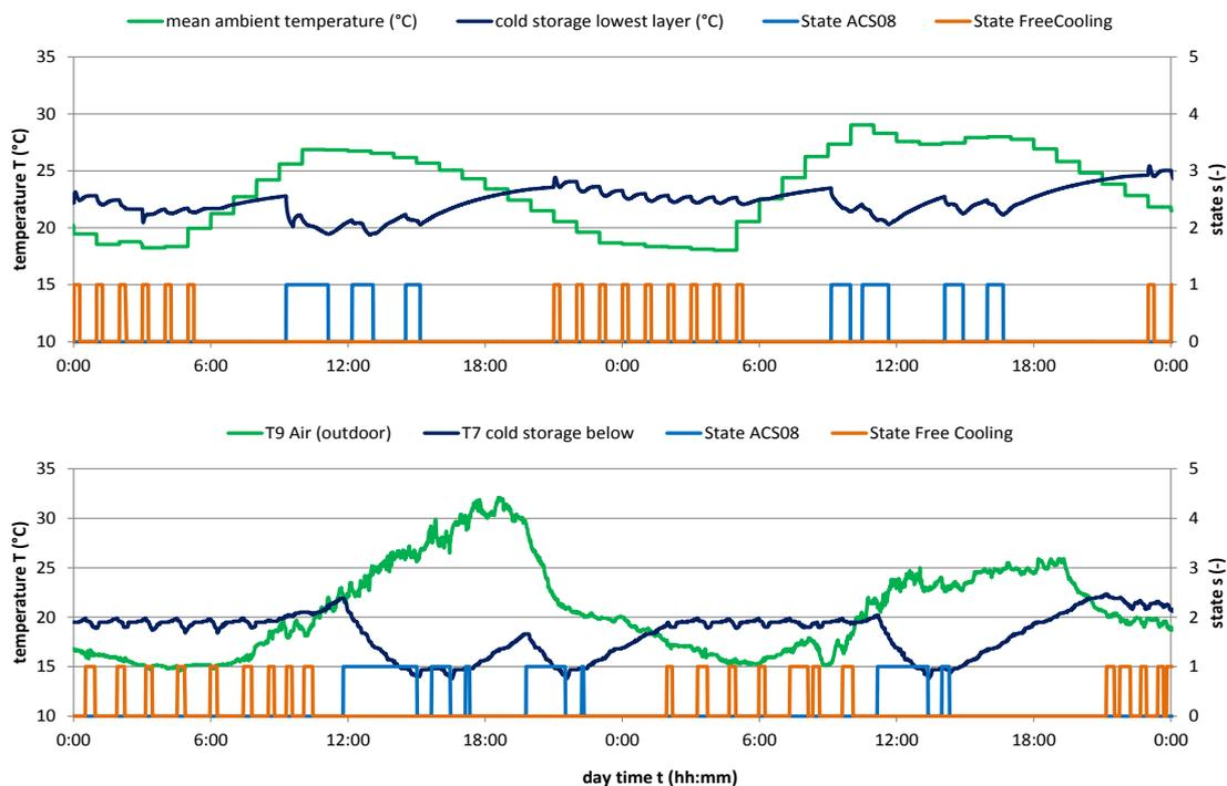
Figure 5: Ambient temperature at the location and temperatures in function of time in the cold storage (lowest layer) as well as the states of the cooling machine ACS08 and the free cooling (ON=1 & OFF=0) in the simulation (above) and in the measurement (below).
