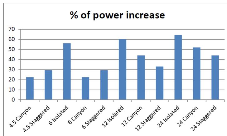
Figure 4 Comparison between the increase in the energy yield of the proposed wind turbine
