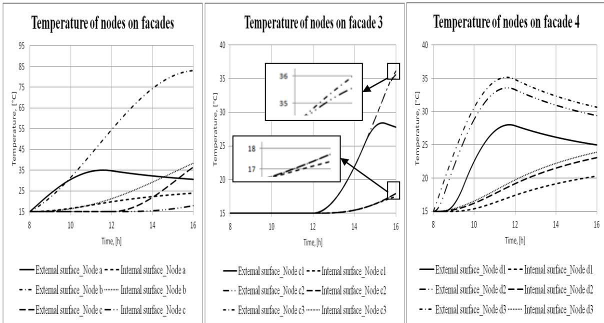
Figure 5: Temperature of central nodes on facades
