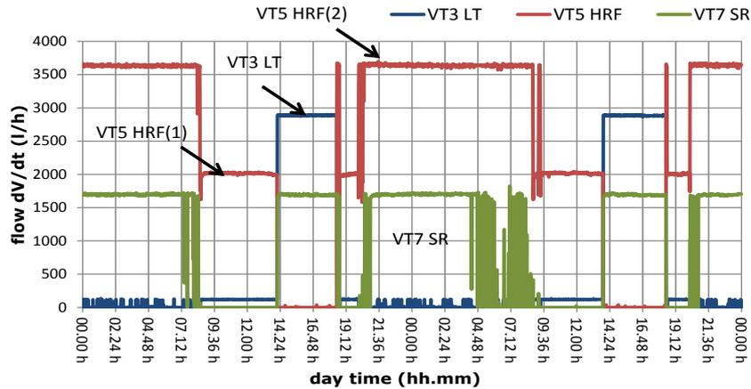
Figure 2: Volume flow data from the solar thermal driven 8kW ACS08 cooling machine. In the simulation environment of POLYSUN the three different flows in VT3 LT, VT5 HRF(1) and VT5 HRF(2) will be realised with two different pumps and a programmable controller. For the nomenclature of VT3 LT, VT5 HRF and VT7 SR see Figure 1.
