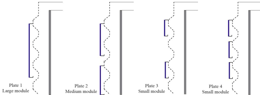
Figure 2: Sketch of different PV module dimensions mounted on UTCs
