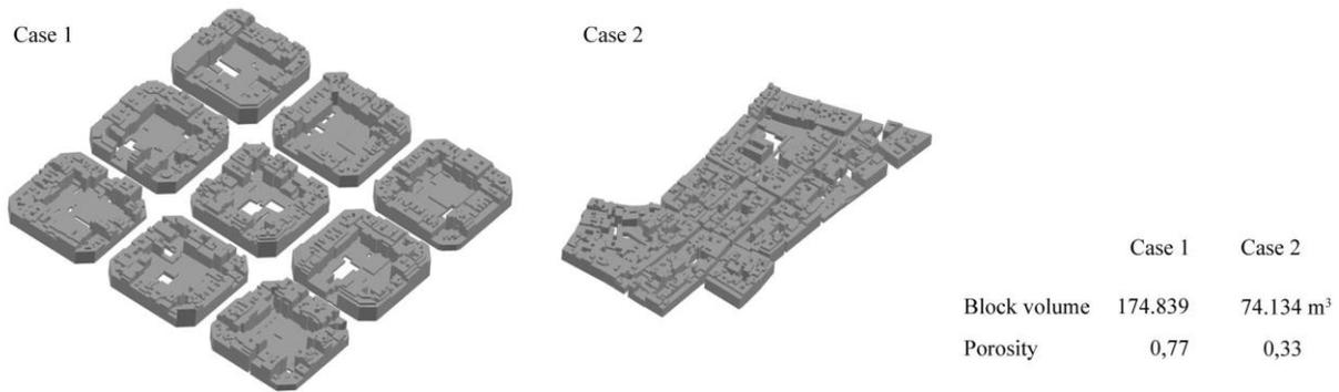
Figure 2: Morphological models of the Eixample (left) and Barri Gotic samples (right)
