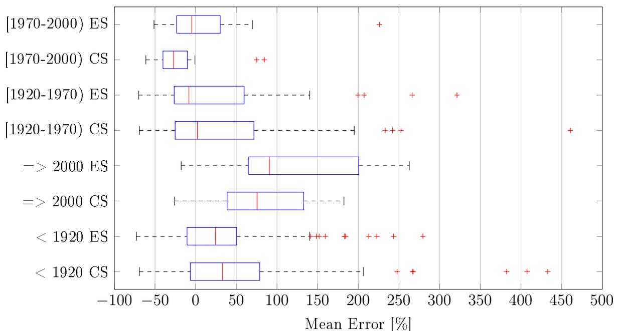
Figure 1: La Chaux-de-Fonds: Boxplot of the error between measurement and estimation with either the energetic signature(ES) or CitySim(CS) for different construction periods.
