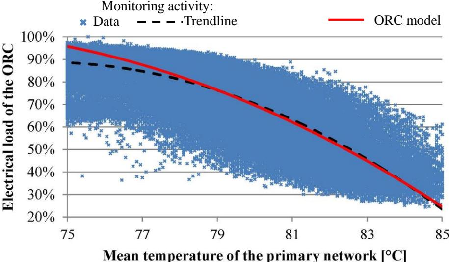
Figure 3: ORC electrical load depending on the mean temperature of the primary network.
