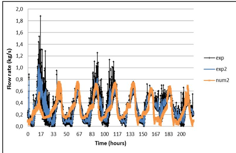
Figure 3: measured and calculated air flow rate during 9 consecutive days in June (summer). Data series “exp” and “exp2” refer to instantaneous and moving average values respectively.
