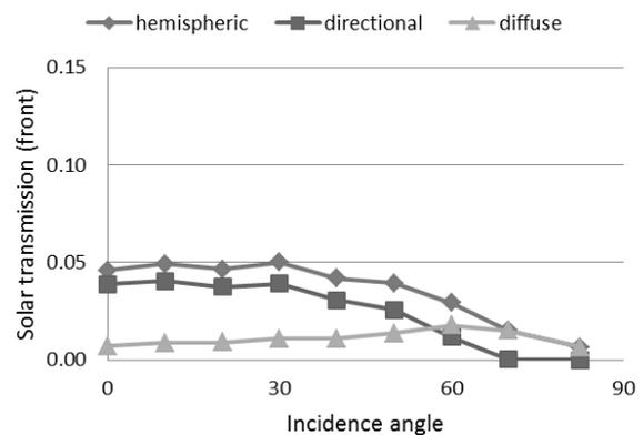
Figure 3: Hemispheric Front Solar Transmittance of Sc2
