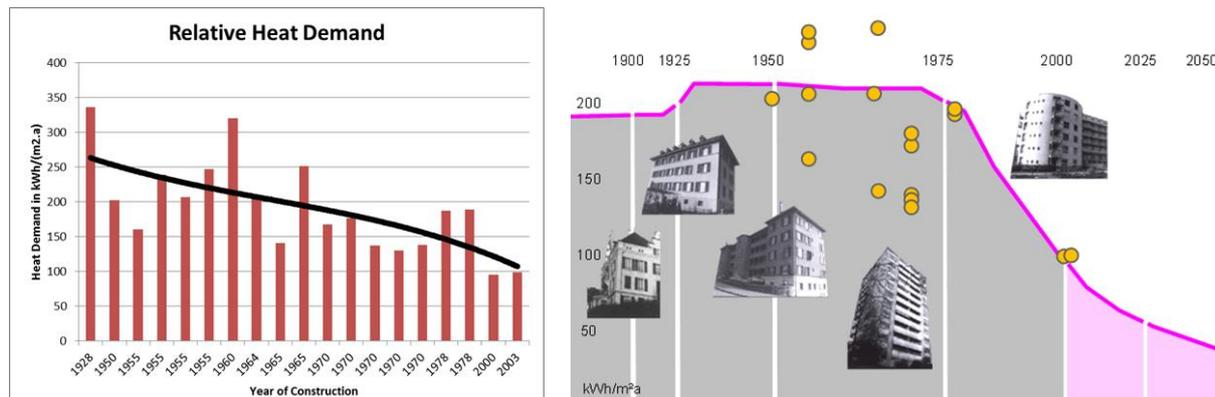
Figure 3: Evaluation of the simulation with the average annual specific energy demand with respect to the construction year based on [5]
