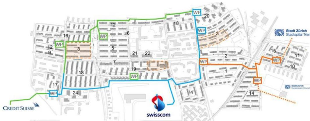
Figure 1: Overview of the planned low temperature network by construction phases. Blue: first construction phase, green: second construction phase, orange: third construction phase. Energy canters with heat pumps are marked with WP. (The coloured graph only available in the digital version of the paper)
