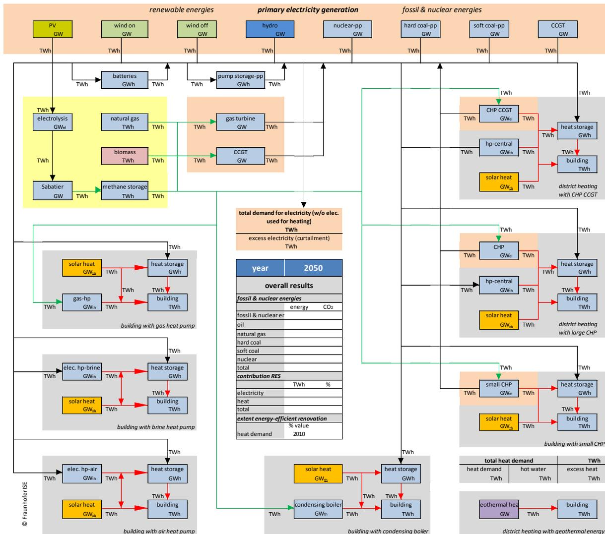
Figure 1: Topology of the model of the German energy system (electricity and heat sector) of the REMod-D model
