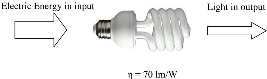
Figure 1 – Efficiency of a common compact fluorescent lamp
