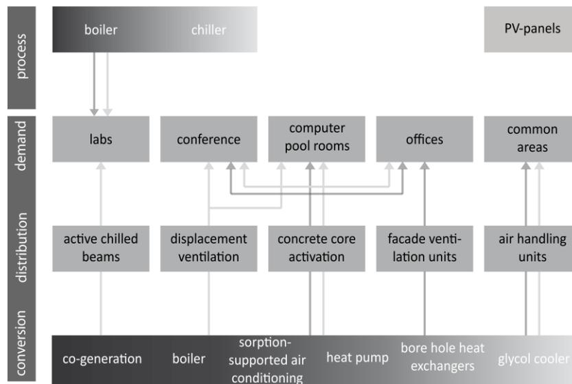
Figure 1: Energy concept of the monitored multifunctional office building.
