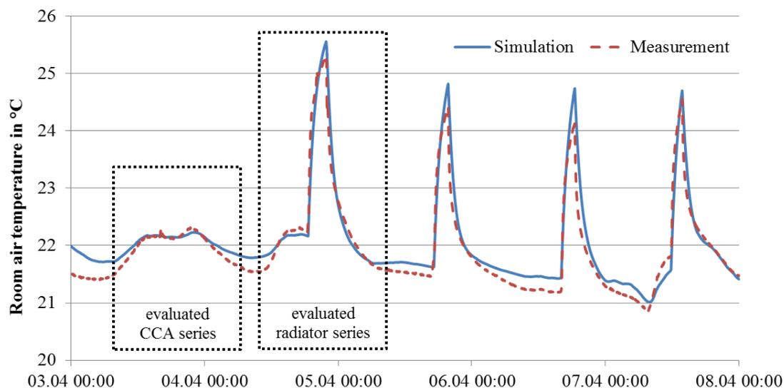
Figure 1: Comparison between simulation and measurement for the room air temperature
