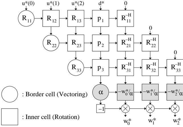
Fig. 4 A systolic array for the production of a 3-tap weight vector using Extended QRD-RLS. Border cells doing complex vectoring and inner cells doing complex rotation are represented respectively as round and squared cells. A distinction is made between cells that must apply the forgetting factor, in white, and the ones that don't, in gray.
