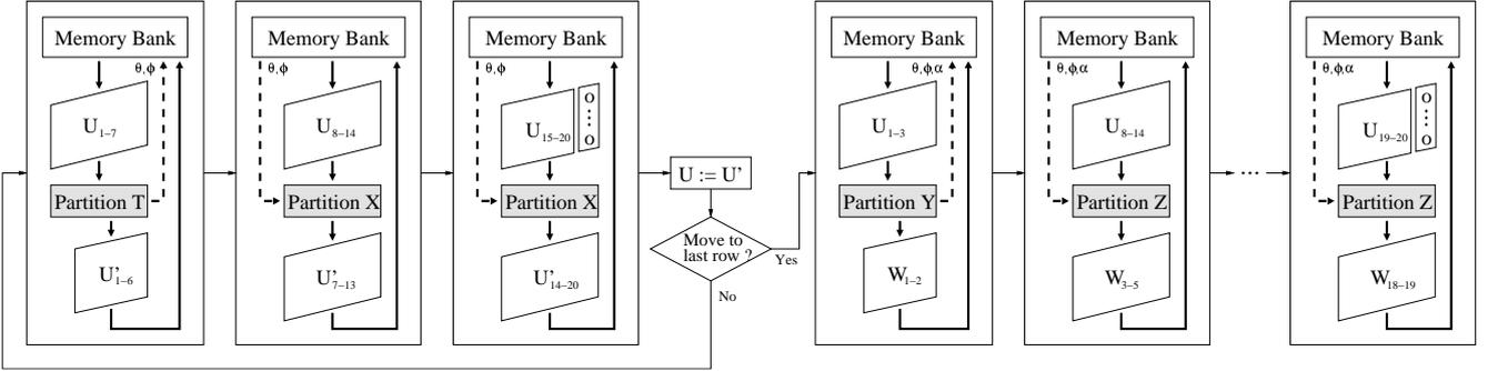
Fig. 8 A run of the algorithm for a 19-tap weight vector. The gray rectangle represents the array of CORSAEngine, the dashed line is for angles and scaling factor that return to memory.  $U_{i-j}$  is the matrix composed of the  $i^{\text{th}}$  to the  $j^{\text{th}}$  columns of  $U$ . The matrix  $W$  output by the last row contains all the weight vectors produced by the processing of the matrix  $U$  through the Extended QRD-RLS systolic array.
