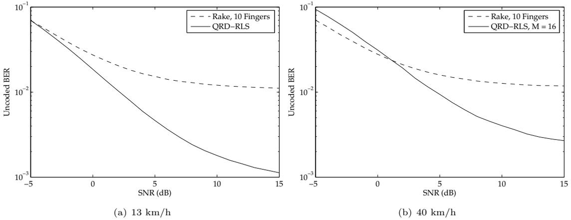
Fig. 9 Performance of QRD-RLS in quarter system load (4 users) with a spreading factor of 16.
