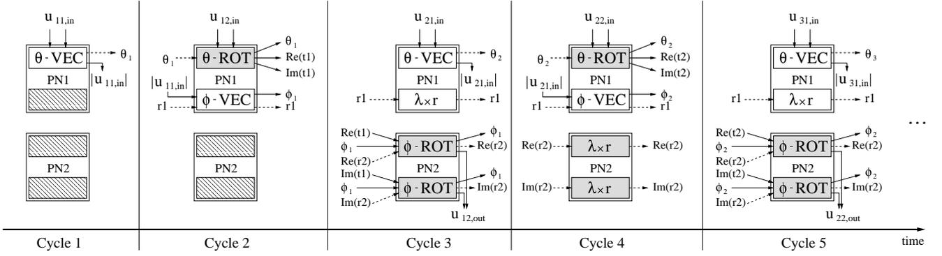
Fig. 6 An example of a border (vectoring) and an inner (rotation) cell on a normal row sharing a CORDIC respectively for the vectoring and rotation of their inputs. The CORDIC is used in vectoring mode during the odd cycles and in rotation mode during the even cycles. Dashed lines represent values that are kept in a register.
