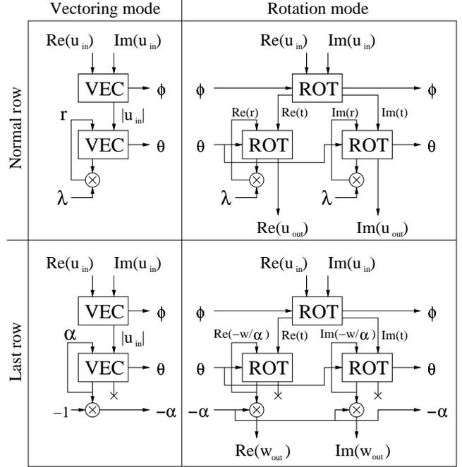
Fig. 5 The CORDIC implementation of the different cells composing a systolic array for Extended QRD-RLS. The multiplication present are also implemented with CORDIC units using a multiplication opcode. the values  $r$  and  $\lambda$  are contained in the registers of the CORDIC units.
