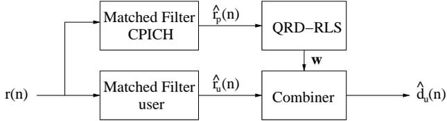
Fig. 2 Block diagram of WCDMA receiver based on QRD-RLS.
