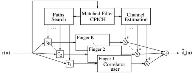
Fig. 1 Block diagram of the conventional RAKE receiver.
