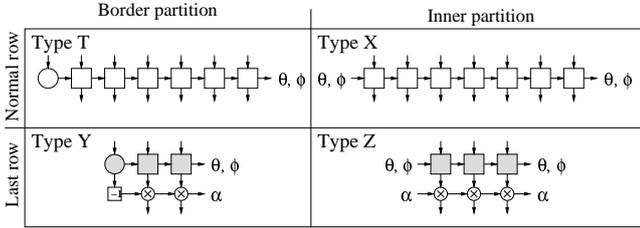
Fig. 7 The four partition types created. With those four types, it is possible to process different array size on the same rectangular systolic array.
