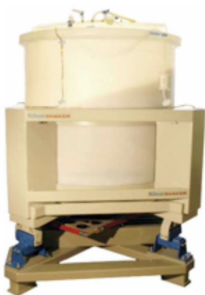
Figure 1.1: An orbitally shaken reactor with both the container and the shaker displayed.
