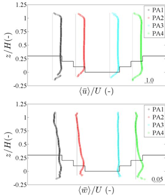
Figure 9 - Up: double average (DA) longitudinal velocity profiles; Down: DA vertical velocity profiles. Black line stands for relative stem density
