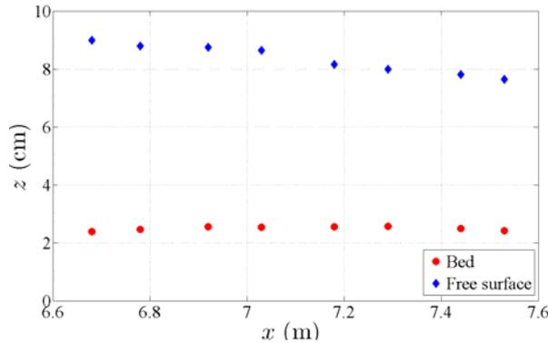
Figure 3 - Longitudinal profile of bed and free surface level.
