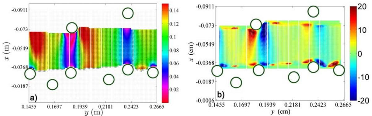
Figure 6 - Horizontal mean velocity (a) and vorticity (b)) at position P3.
