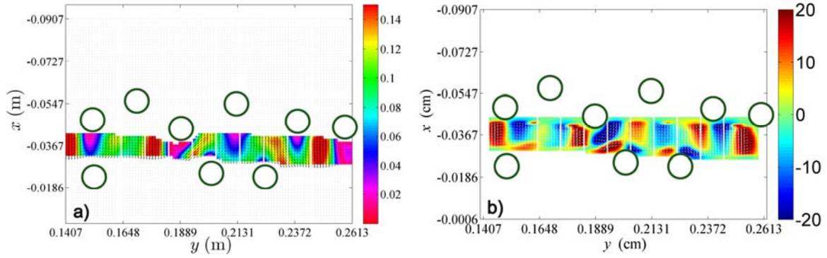
Figure 4 – a) Horizontal mean velocity map (m/s) at P1; b) vorticity map ( $s^{-1}$ ) based on mean flow field at P1. Circles represent the nearest stems and the vertical white lines indicate the lateral positions where the vertical measurements were acquired. In these graphs,  $x$  represents a local reference for the flow direction and  $y$  stands for the transversal coordinate indicating the distance to the right side wall of the flume. The longitudinal position P5 presents a similar result.
