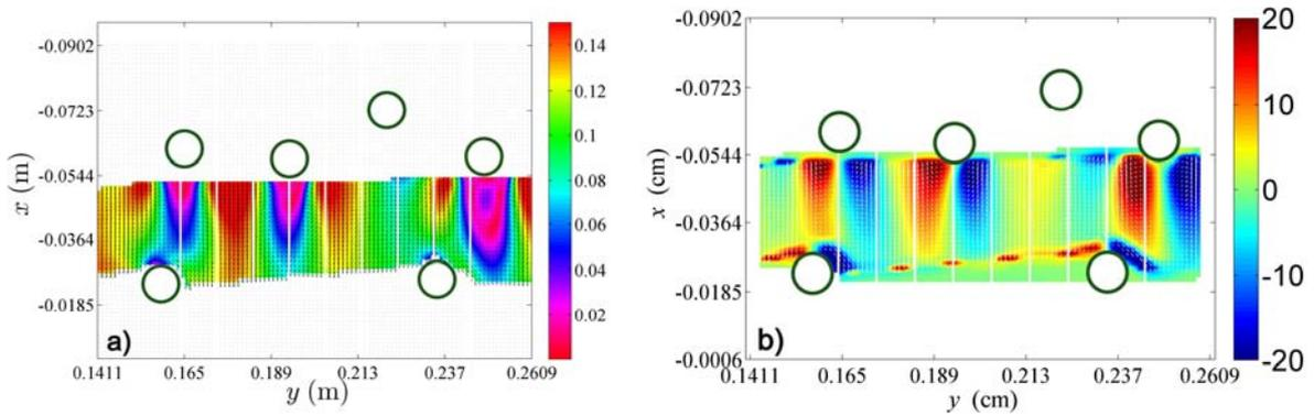
Figure 5 – Horizontal mean velocity (a) and vorticity (b)) at position P2.
