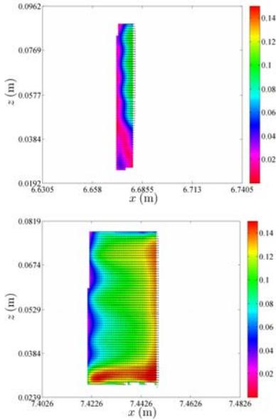
Figure 8 - Examples of vertical velocity fields. Left: P1 at  $y=19.4$  cm; right: P7 at  $y=21.4$  cm (cf. Fig.2 for the location of profiles).
