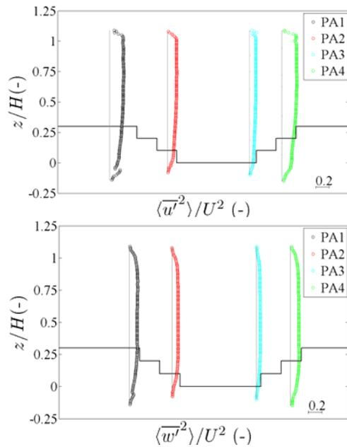
Figure 12 - DA Reynolds normal profiles: up: longitudinal; down: vertical.
