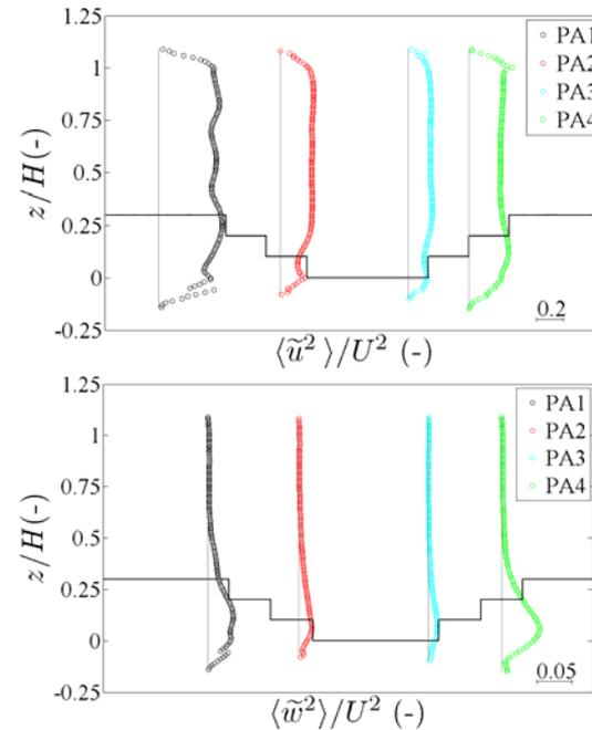
Figure 11 - DA form-induced normal profiles: up: longitudinal; down: vertical.
