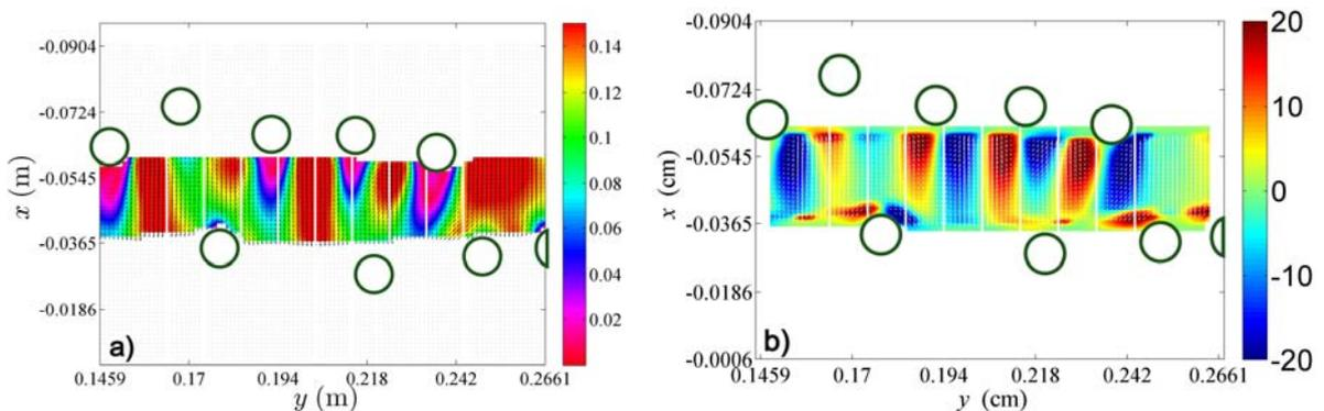
Figure 7 - Horizontal mean velocity (a) and vorticity (b)) at position P4.
