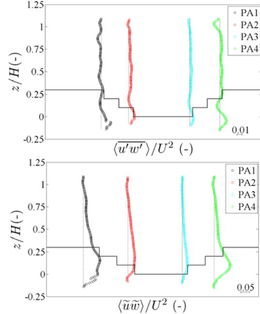
Figure 10 - DA shear stress profiles: up: Reynolds; down: form-induced.
