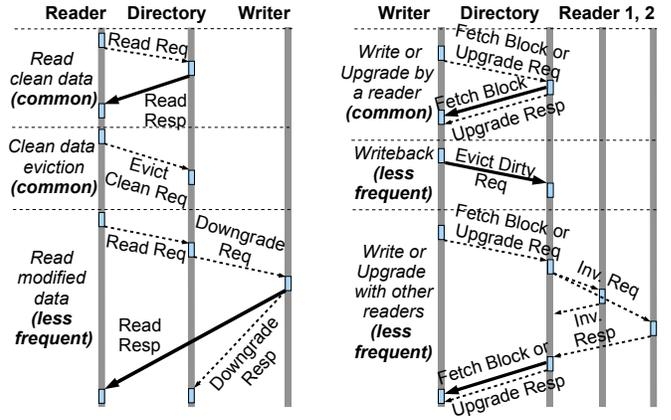
**Figure 2:** Read (left) and Write (right) protocol activity.
