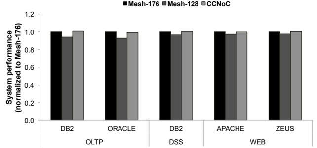
**Figure 7:** System performance (User-IPC) normalized to Mesh-176.
