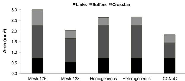
Figure 11: NoC area for various network topologies.
