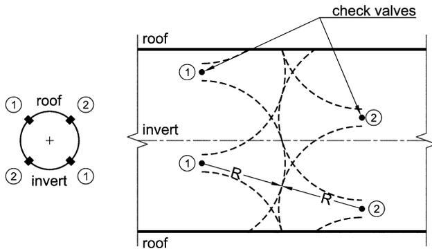
**Fig. 6** Cross-section of steel liner equipped with pressure relief valves (*left*). Radial symmetric seepage flow towards the valves in the unfolded cylindrical gap (*right*). The maximum radial distance  $R$  of the seepage flow towards the check valve corresponds to half of the maximum distance between any two valves
