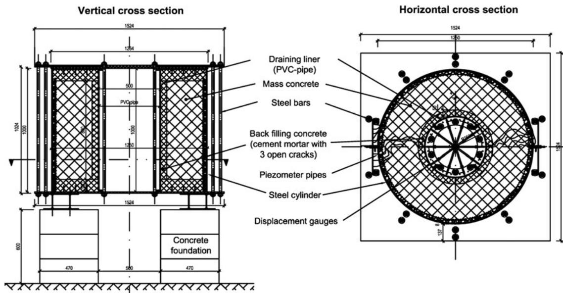
**Fig. 8** Experimental set-up for physical modelling of the steel liner drainage system with different pressure relief valve configurations. *Left* vertical cross-section showing the steel pressure vessel with pre-stressed steel bars for stabilizing the bottom and top cap of the cylinder as well as the inner PVC pipe (reproducing the liner)
