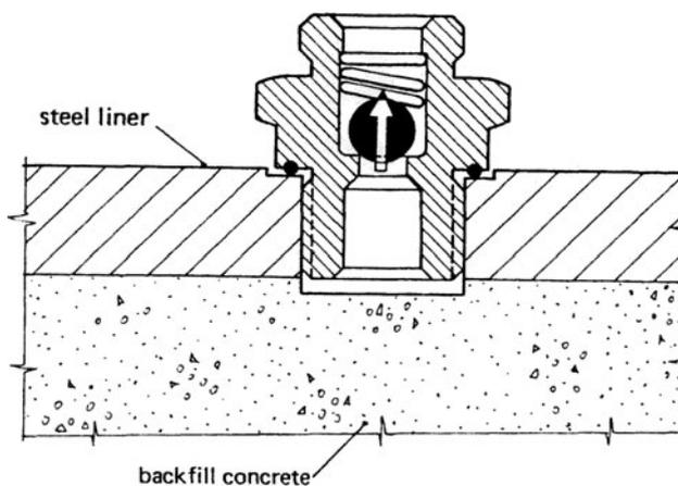
**Fig. 3** Section of the pressure relief valve installed in the steel liner of the Collierville tunnel; the diameter of the valve orifice is 20 mm
