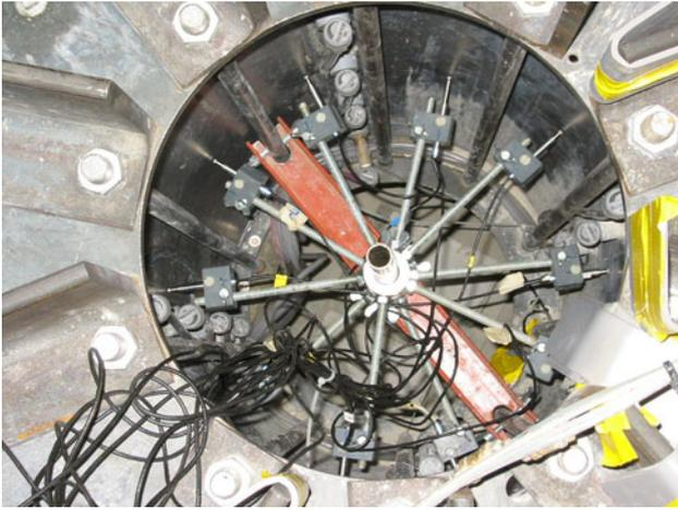
**Fig. 9** Top view inside the PVC pipe representing the liner, in which radial deformation is measured with 10 long-base extensometers. The opening and closing wheel of the valves can also be seen
