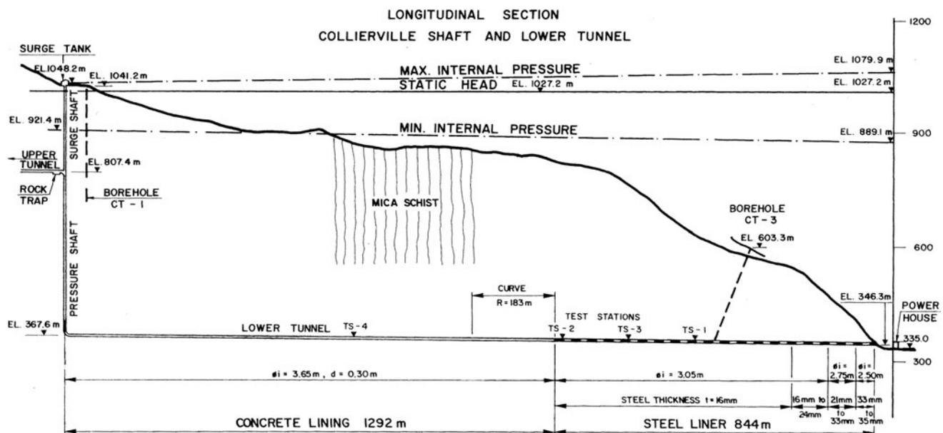
**Fig. 2** Longitudinal section of the Collierville shaft and lower high-pressure tunnel of the North Fork Stanislaus River Hydroelectric Power Plant in California. Locations of boreholes (CT-1 and CT-3) and hydraulic fracturing tests (TS-1 to TS-4) are also shown
