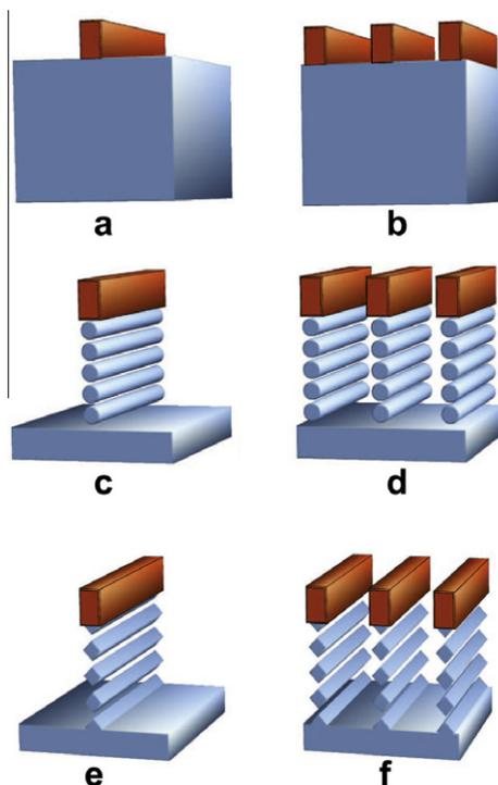
**Fig. 1.** Fabrication flow. (a) Single HSQ line patterned on Si substrate. Typical HSQ width is 50 nm. (b) Dense HSQ line arrays. (c and d) After etching with recipe (2) as reported in Table 3. (e and f) After etching with recipe (3) as reported in Table 3.
