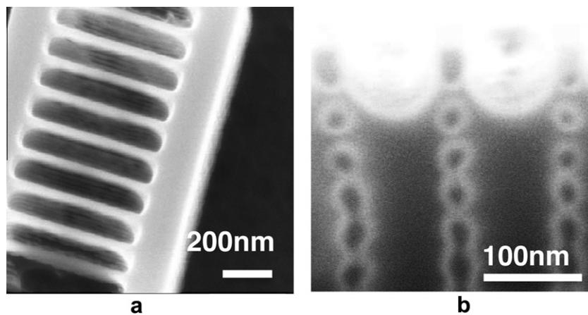
**Fig. 6.** Examples of dense nanowire arrays. Etching parameters are  $200\text{ cm}^3/\text{min}$  and 2.5 s for  $\text{SF}_6$ ,  $150\text{ cm}^3/\text{min}$  and 1 s for  $\text{C}_4\text{F}_8$ . (a) Bird's eye view of a 550 nm long wires with 200 nm pitch cut with FIB. (b) Cross-section for an array with 300 nm long wires and 100 nm pitch. The average nanowire diameter is 25 nm.
