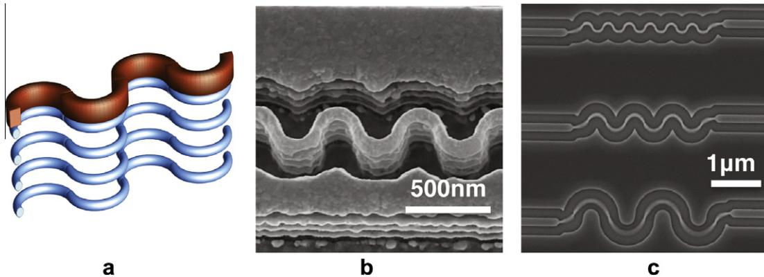
**Fig. 3.** (a) Concept view of vertically-stacked curved nanowires. Etching parameters are  $200 \text{ cm}^3/\text{min}$  and 2.5 s for  $\text{SF}_6$ ,  $150 \text{ cm}^3/\text{min}$  and 1 s for  $\text{C}_4\text{F}_8$ . (b) Bird's eye view of the nanowire stack covered by a 50 nm thick Pt layer for conformal PtSi silicide formation. (c) Top view of the three curved nanowire design.
