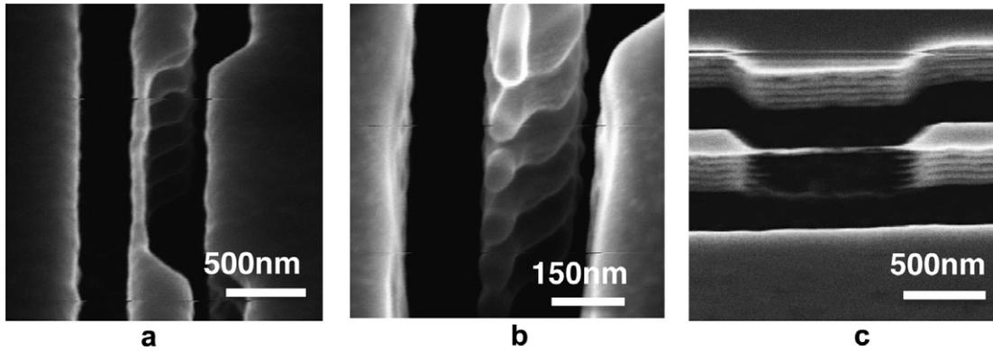
**Fig. 2.** Vertically stacked 50 nm diameter for straight-line nanowires carved inside a 200 nm narrow trench. (a) Bird's eye view. (b) Cross-section. The etching parameters are  $300 \text{ cm}^3/\text{min}$  and 3 s for  $\text{SF}_6$ ,  $150 \text{ cm}^3/\text{min}$  and 1 s for  $\text{C}_4\text{F}_8$ . (c) Tilted view of a straight-line nanowire stack carved in a 500 nm wide trench. Due to a reduced etchant depletion effect, all the nanowires but the top one are overetched.
