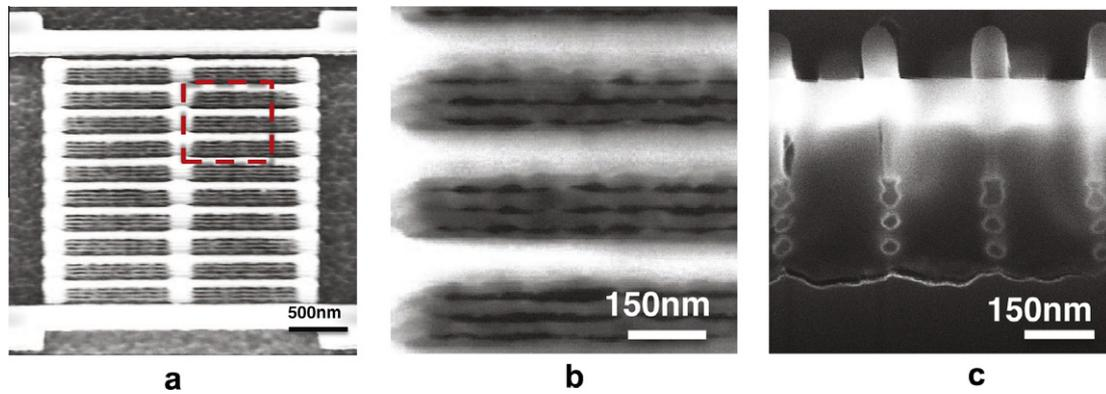
**Fig. 5.** Examples of nanowire arrays with 200 nm pitch,  $\mu\text{m}$  length and 30 nm average diameter. Etching parameters are  $200\text{ cm}^3/\text{min}$  and 2.5 s for  $\text{SF}_6$ ,  $150\text{ cm}^3/\text{min}$  and 1 s for  $\text{C}_4\text{F}_8$ . (a) Bird's eye view. (b) High magnification showing the vertical stacks. (c) Cross-section of the vertically stacked array.
