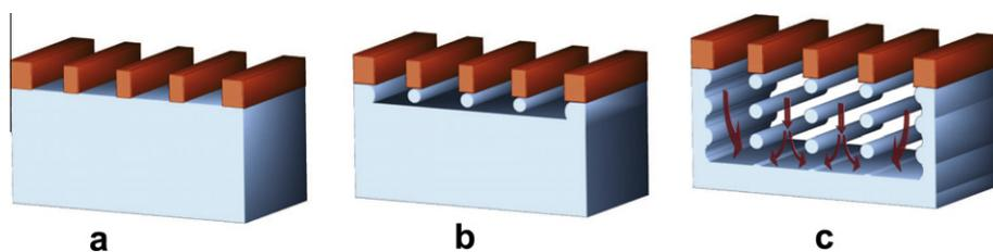
**Fig. 4.** (a) Dense array before etching. (b) Nanowire formation at etching time step  $t_1$ . (c) After  $4 \cdot t_1$  3 levels of SiNWs are obtained and a fourth one begins to form. The arrows indicate the plasma flow directions.
