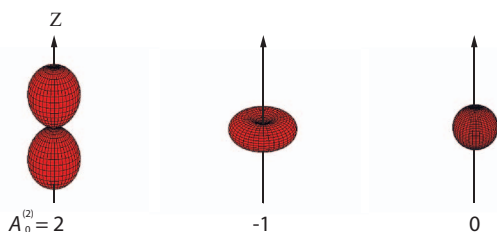
FIG. 3. Angular distributions P_J(\theta) for different values of the angular momentum alignment coefficients A_0^{(2)} = 2, -1, \text{ and } 0 .
