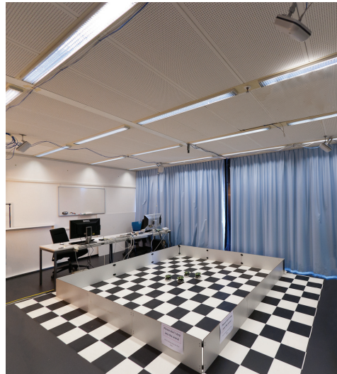
Fig. 2. Experimental setup in the laboratory space. The UWB base-stations are mounted on the ceiling above the extremities of a 9m 2 robotic arena, and an overhead camera is mounted on the ceiling above the center of the arena.
