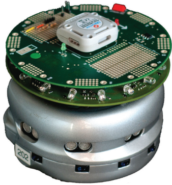
Fig. 7. The Khepera III robot is equipped with an extension range and bearing module which utilizes sixteen evenly-spaced infrared Light Emitting Diodes (LEDs). On top of this board, we mounted an active marker (LED) tracking module which simultaneously carries the Ubisense tag.
