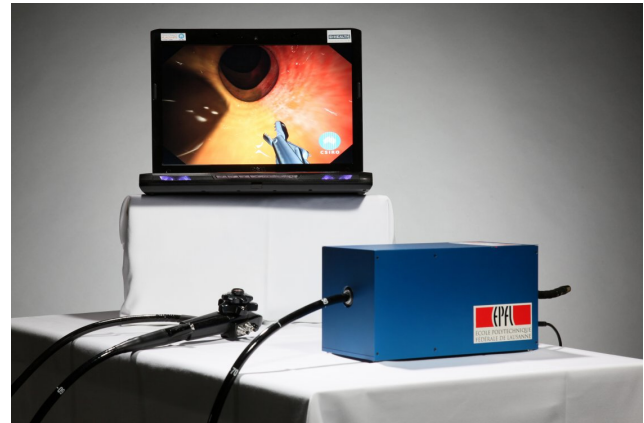
Figure 1: The colonoscopy simulator consists of a 2-DOF haptic interface, an instrumented clinical endoscope and a virtual reality environment to provide real-time visualization.
