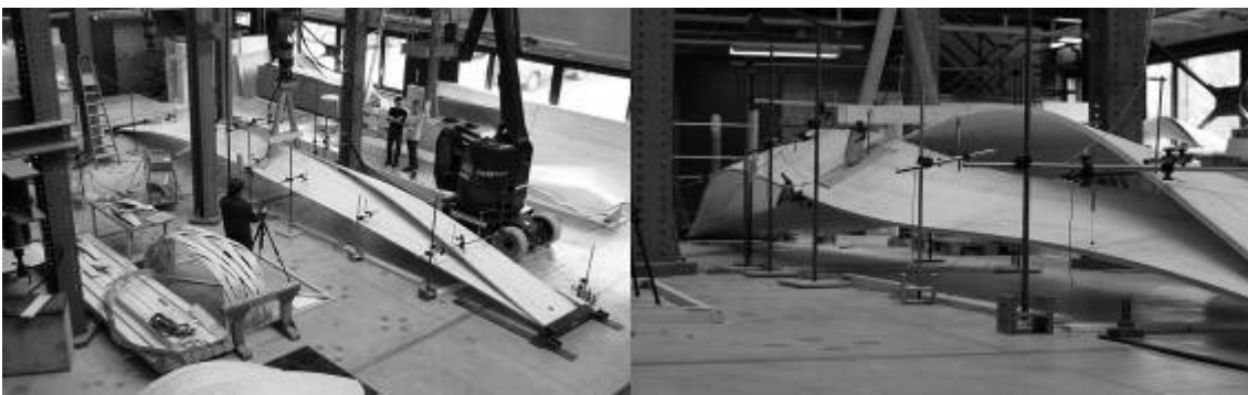
Figure 6. Real scale testing on textile modules
