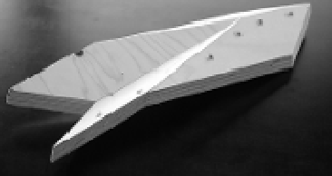
Figure 2. Prefabricated timber element; real scale prototype
