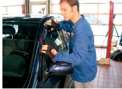
Figure 2. Car manufacturing scenario. Seven IMU sensor nodes are located on the body during recording data, [11].
