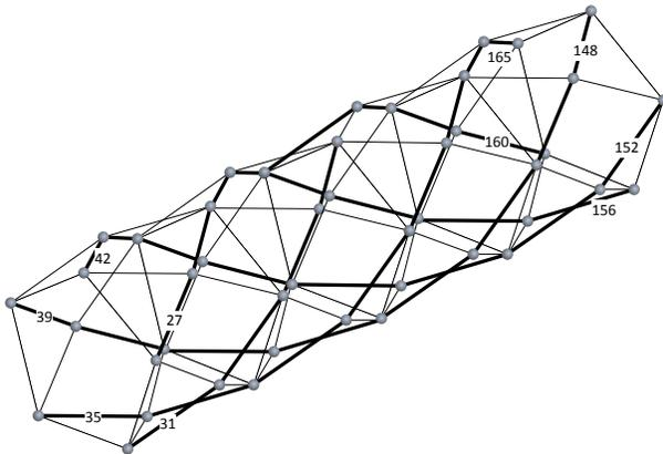
**Figure 13.** Active cables in Group 1 with CCC
