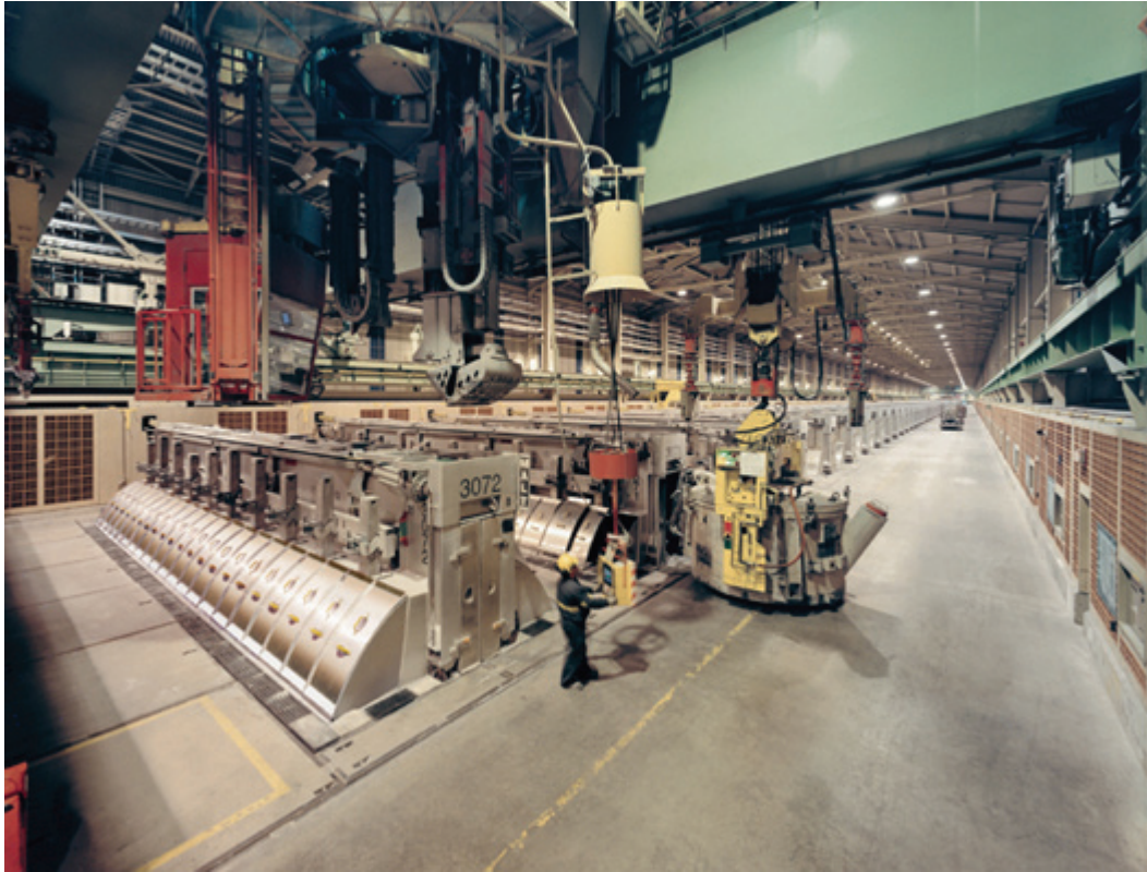
Figure 3: View of a potroom. Siphoning of aluminium is done at the right. Photo Courtesy of Rio Tinto Alcan.
