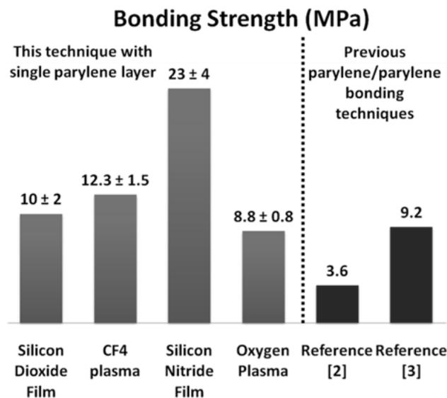
Figure 5- Results of the pull-test measurements for different cases and comparison with existing parylene/parylene bonding techniques. For this study, each bar corresponds to mean of at least 6 experiments. For comparison, anodic bonding results in a bonding strength around 30-40 MPa depending on the bonding temperature [1].
