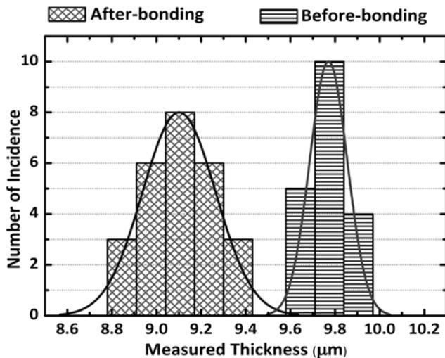
Figure 3 – Histogram of parylene-C thickness measurements before and after the bonding, obtained from cross-section observations. Before bonding, measurements indicate a thickness of  $(9.77 \pm 0.07) \mu\text{m}$ , while after bonding a thickness of  $(9.10 \pm 0.16) \mu\text{m}$  is observed, corresponding to a 7% thickness reduction on average.
