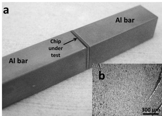
Figure 4 – Bonded samples for pull-testing. (a) Assembly of sample with aluminium pulling bars. (b) Optical microscope image of fractured interface after pull-testing. In general, fracture occurs in the form of cracks within the parylene-C layer.
