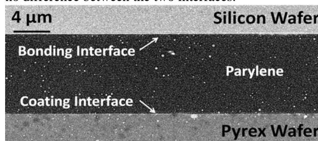
Figure 2 – SEM image of a cross-section of the bonding stack and the parylene-C/Si bonding interface. Cross-sections of the bonding stack were realized by dicing the wafers, followed by polishing and thermal evaporation of a 20 nm thick carbon layer for SEM observation. Other bonding combinations also show no difference in bonding quality between the two interfaces.
