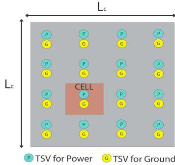
Figure 1. PDN top view-Placement of the TSVs.
