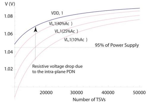
Figure 5. The voltage on the top and first metal layers of the plane located the farthest from the package pads for constant TSV diameter ( $5 \text{ }\mu\text{m}$ ) and varying TSV number is illustrated.
