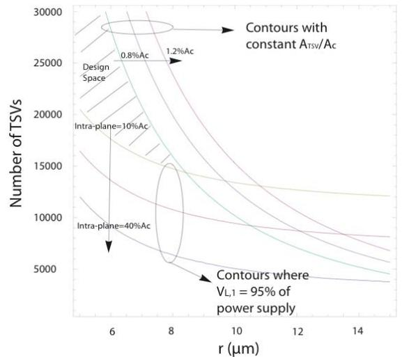
Figure 6. Design space defined by the contour plots  $V_{L,1} = 0.95V_{Power\_Supply}$  and  $(A_{TSV}/A_c) = \text{constant}$ . This design space varies as a function of the area
