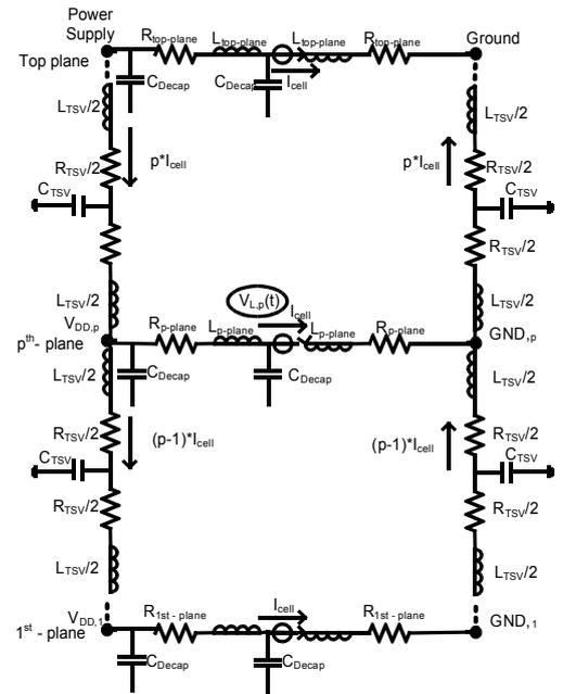
Figure 3. The equivalent RLC model describing the PDN of a cell.
