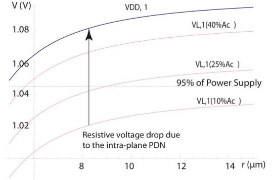
Figure 4. The voltage on the top and first metal layers of the plane located the farthest from the package pads for constant TSV number (10K) and varying TSV diameter is illustrated.
