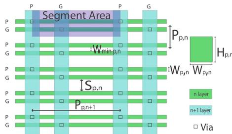
Figure 2. Top-view of the intra-plane power distribution network.
