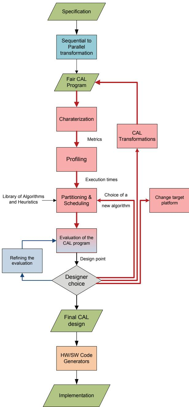
**Fig. 1:** Design Flow: interlacing of a design and an evaluation loops.
