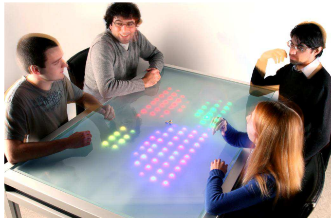
Fig. 1. The current design of Reflect with color-coded circles around each speaker position indicating how much the person has spoken.
