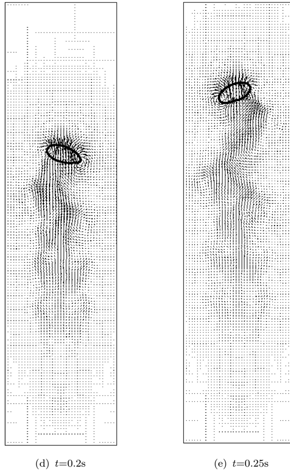
Figure 5.29: Interface position and velocity field with 3D CLSVOF for 5mm bubble, cont.
