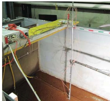
Figure 3: The  $5 \times 5$  UVP-transducers rack fixed on the vertical stem with its remote computer installed on the bridge.
