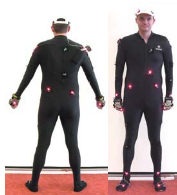
Fig. 5. reduced set of marker used for the real-time full-body interactions
