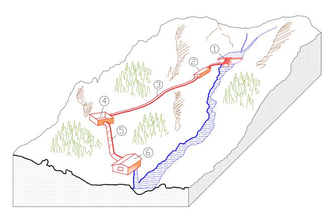
Figure: Main component of a high-head SHP plant (Andaroodi, Schleiss et al., 2005, p. 22)
