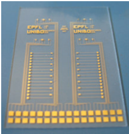
Fig. 2: Micro-fabricated chip used to investigate the different DNA probe immobilizations showed in Figure 1.
