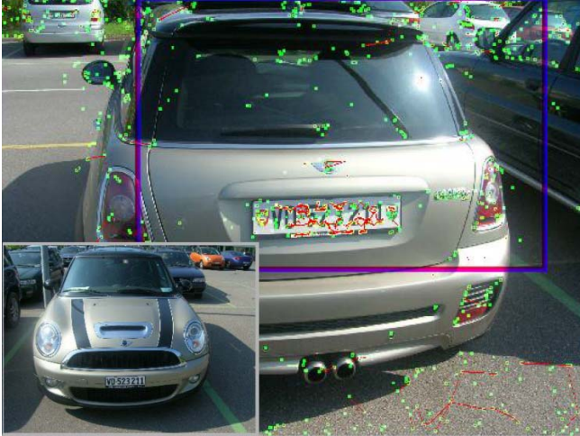
Figure 11. Object duplicate detection algorithm detected the back side of a car, thanks to the license plate. Training image is on the bottom left corner.
