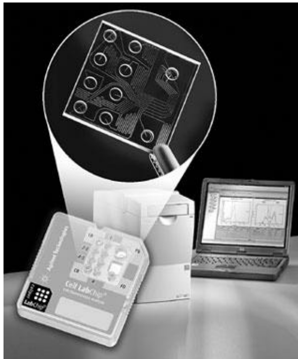
Figure 1-3 example of a Lab-on-Chip device: Agilent 2100 Bioanalyzer, together with its Cell Assay Extension, can perform simple flow-cytometric analysis.
