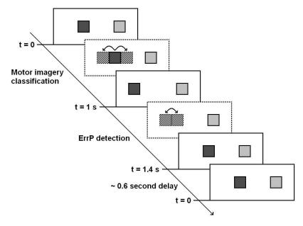
Figure 1: Timing of the protocol. At t=0, the target is 3 steps on the right of the cursor. At t=1 second, the system makes a mistake and moves the cursor to the left while the subject was imagining a movement of his right foot. At t=1.4 second, the system detects ErrP and cancels the wrong movement. After a delay of about 600 ms, the system starts accumulating data for the next motor imagery classification, i.e. for the next single trial.
