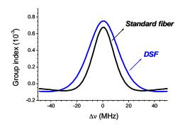
Fig. 2-(a) Group index variation according to frequency deviation from Brillouin frequency. The gain is 20dB when  $\Delta v = 0$
