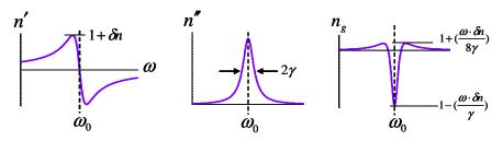
Fig. 1. Relation between the phase constant (n'), the attenuation constant (n'') and the group index  $(n_g)$  around the absorption peak centered at  $\omega_0$ .
