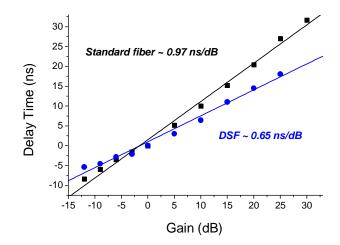
Fig. 5. Delay time of the pulse as a function of the Brillouin gain. In a gain situation the pulse is delayed while it is accelerated in a loss configuration.
