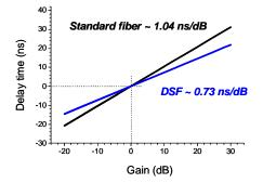
Fig. 2-(b) Delay time as a function of Brillouin gain..
