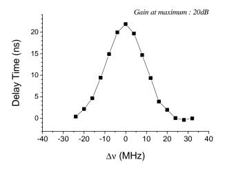
Fig. 6. Delay time of the probe pulse as a function of the modulation frequency deviation ( $\Delta \nu$ ) from  $\nu_B$ . The pump and the probe powers were fixed.
