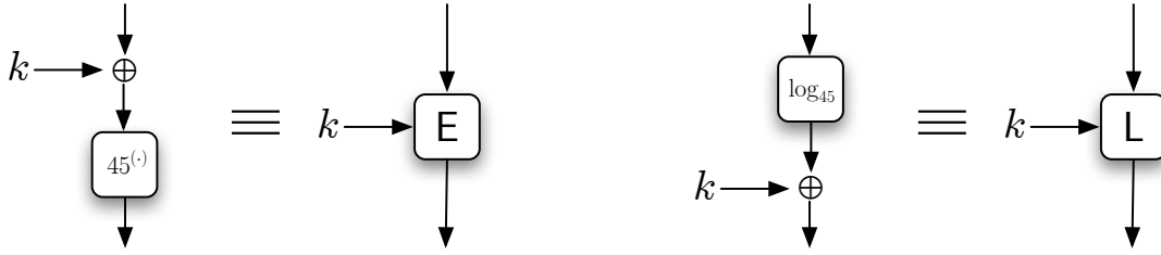
Figure 9.2: Replacing key exclusive-or and fixed substitution boxes by equivalent keyed substitution boxes
