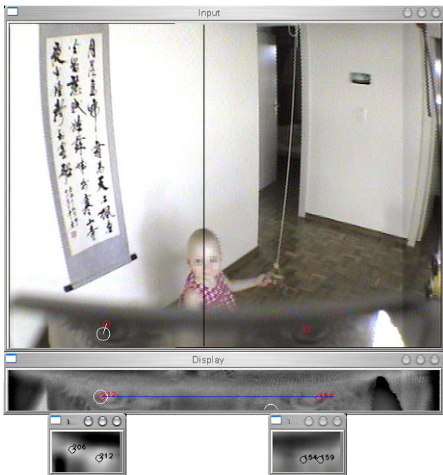
Fig. 11. Detection of the gaze direction. (top) The eyes of the wearer are reflected in the bottom portion of the WearCam image, the black line shows the estimated direction of the gaze. (middle) Result of the illumination normalization. (bottom) Results of the eye template matching with best candidates. The white and red circles superimposed to the top and middle images show respectively the center of the eyes and the detected position of the pupil in the eye.
