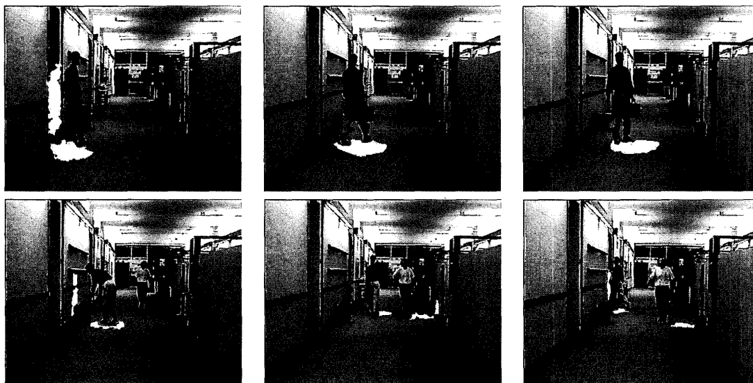
Figure 9: Shadow detection results for sample frames of the test sequence Hall Monitor
