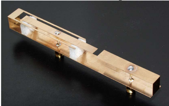
Figure 3 : double PIFA for GSM/DCS (feed point to the left) and UMTS bands
