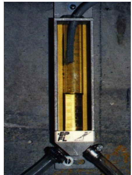
Figure 7: Hydrostatic leveling device with graduated glass container
