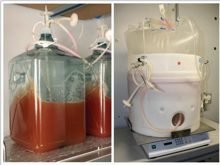
Fig. 5.1. 20-L square-shaped shake bioreactors (left) and 50-L shake bioreactor with a modified benchtop shaker (right).
