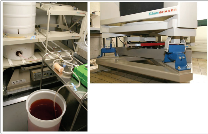
Fig. 4.6. Pilot scale shaker based on a modified RC-X shaker (Adolf Kühner AG, Birsfelden, Switzerland) (left). Production scale prototype shaker designed and constructed by Adolf Kühner AG (right).
