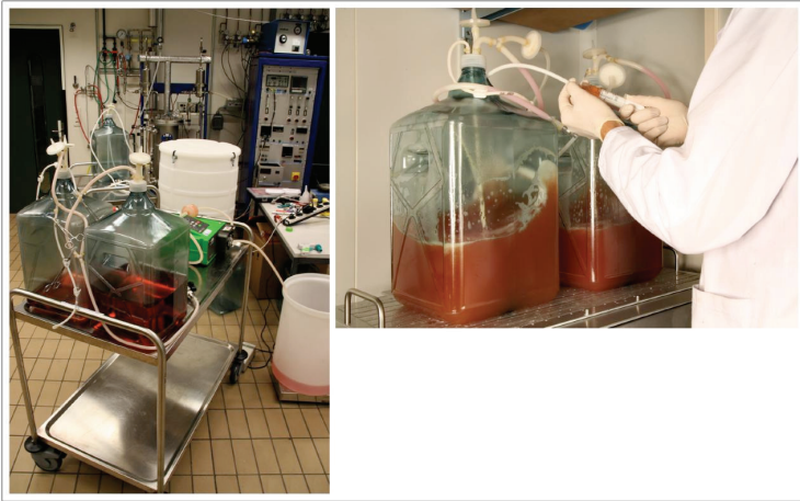
Fig. 4.5. 20-L polycarbonate containers used as disposable shake bioreactors for the cultivation of mammalian cells in suspension. The sterile filtration of the cell culture media (left) and the in situ sampling (right) are shown.
