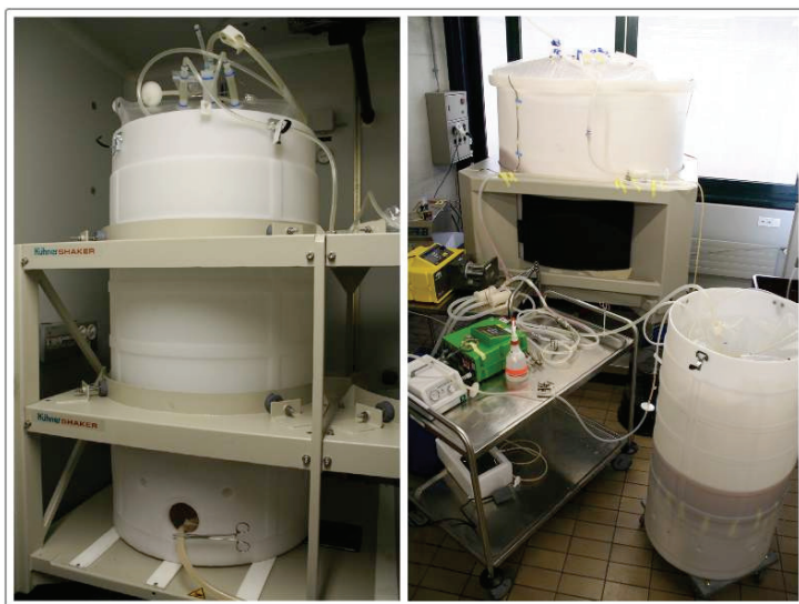
Fig. 4.8. 200-L shake bioreactor and modified large-capacity shaker (left). The production scale bioreactor was inoculated with 75 L of cells expanded using the 200-L shake bioreactor (right).
