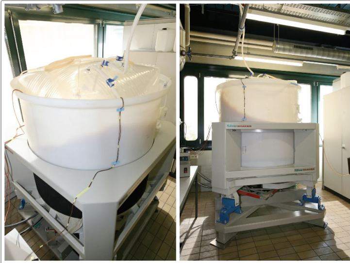
Fig. 4.9. (B) 1'500-L disposable shake bioreactor with a cell culture volume of 750 L and agitated at 43 rpm. Height: 2 m, floorspace: 4 m 2 , weight empty: 1'000 kg.
