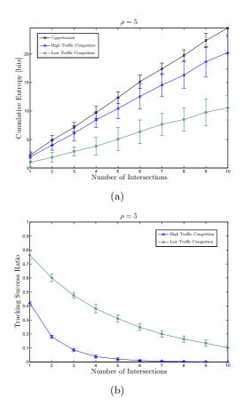
Figure 3: Vehicular Mix-zone simulation results. (a) Location privacy for various vehicle densities. (b) Adversary success probability.
