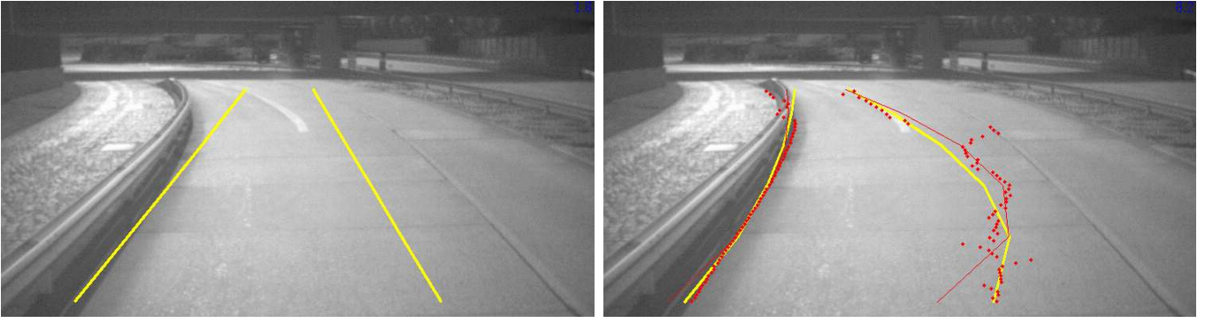
Fig. 2. Lane detection without (left image) and with (right image) cumulated gradient information along the lane. Using this global hypothesis, the algorithm succeeds in situations where the contrast of one street side (left one) is not constant and the other side (right one) has no particular marking.
