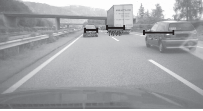
Fig. 3. Typical vehicles detection result. The information of surrounding vehicle is found in the camera coordinate frame, but should be converted in the real 3D space in order to compare the results of the camera module within the fusion step.
